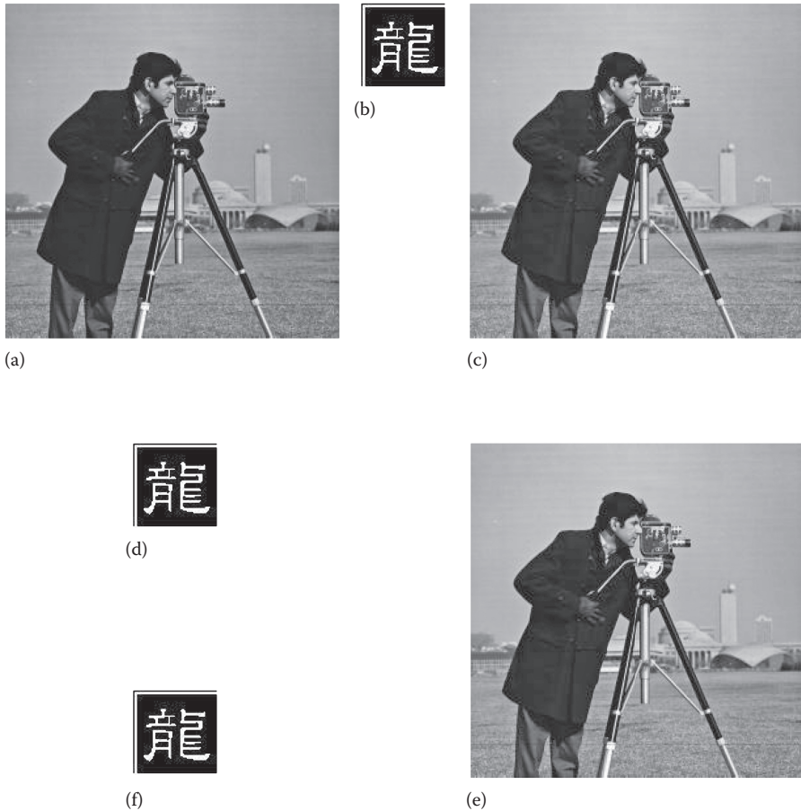
FIGURE 12.14 The images before and after applying the GA and DE algorithms: (a) Cameraman 256 \times 256 cover image, (b) Chinese character 64 \times 64 watermark, (c) Cameraman stego-image after 50 iterations using GA, (d) Extracted watermark from (c), (e) Cameraman stego-image after 50 iterations using DE, (f) Extracted watermark from (e).
