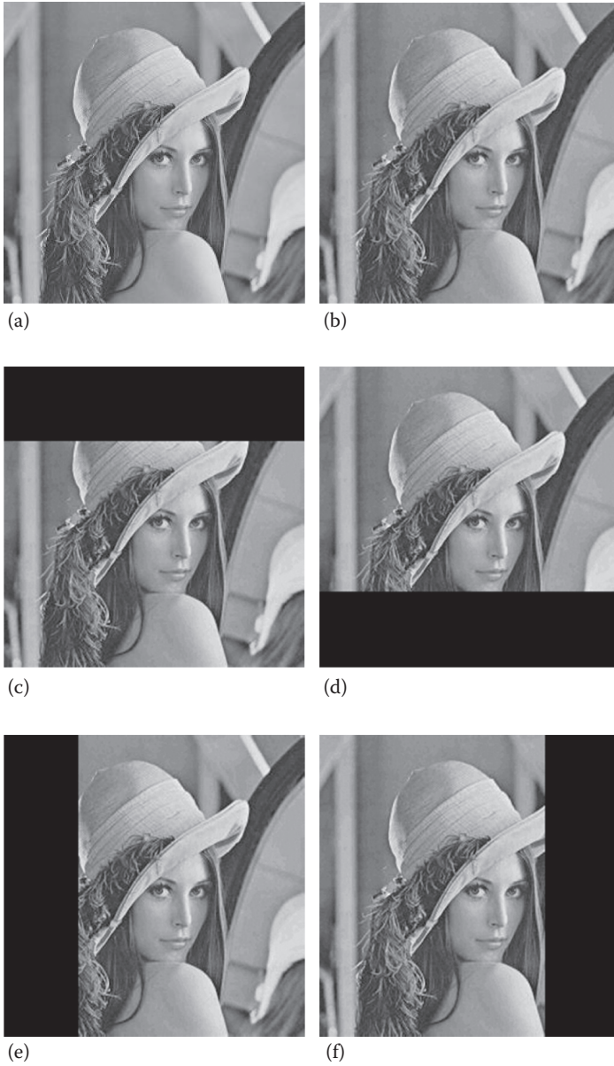
FIGURE 5.25 Different cropping styles: (a) the original Lena 256×256 image, (b) the watermarked Lena image, (c) top 64: cropping 64×256 from the top, (d) bottom 64: cropping 64×256 from the bottom, (e) left 64: cropping 256×64 from the left, (f) right 64: cropping 256×64 from the right.
