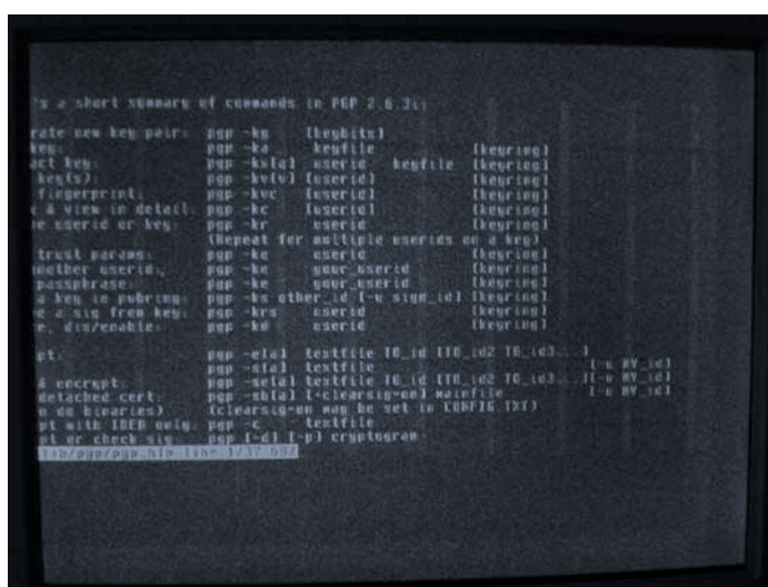
Figure 4.11 Intercepted image of encryption keys using van Eck radiation. (Courtesy of Markus Kuhn and Ross Anderson.)
