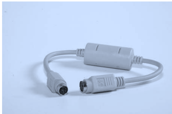
Figure 4.3 Keyghost keystroke-capturing device without adaptors.
