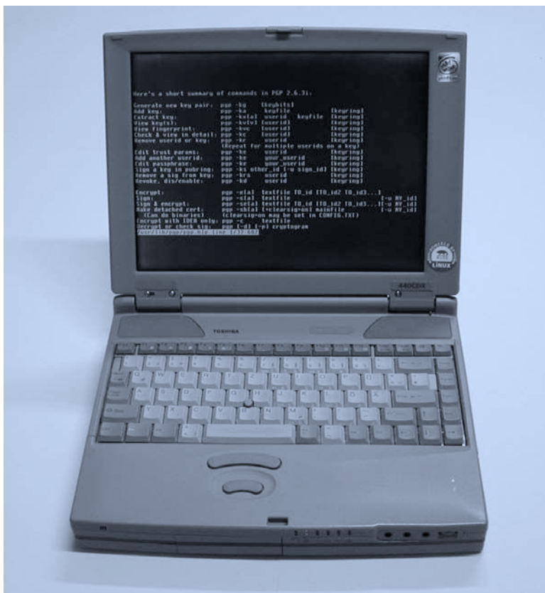
Figure 4.10 Screen display of encryption key setup on targeted computer. (Courtesy of Markus Kuhn and Ross Anderson.)
