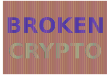
(b) ECB mode ciphertext, 5 pixel (120 bit) block size.
