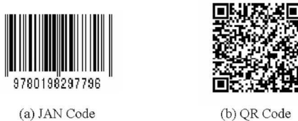
Fig. 10.4. Two examples of bar code, in which (a) is a sample of a 1-dimensional bar codes called JAN Code, and (b) is a sample of a 2-dimensional bar codes called QR Code (Quick Response Code).
