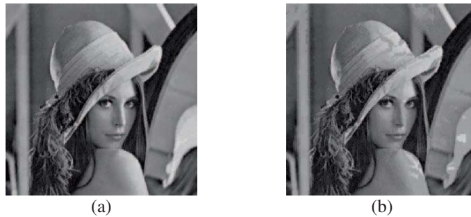
Fig. 11.6. The watermarked images obtained by algorithms having different embedding orders. (a) The watermarked image with PSNR = 30.553 dB obtained by using the proposed method. (b) The watermarked image with PSNR = 26.105 dB obtained by using the algorithm in the reverse embedding order.
