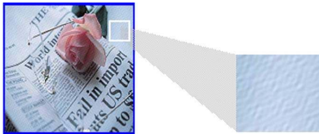
Fig. 10.8. An example of the watermark generated in frequency domain, and the right one is an expanded area in the left image.
