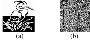
Fig. 11.8. The watermarks extracted from the original image using the two-stage codebooks. (a) Extracted robust watermark, NHS = 1.0 . (b) Extracted semi-fragile watermark, NHS = 0.047 .
