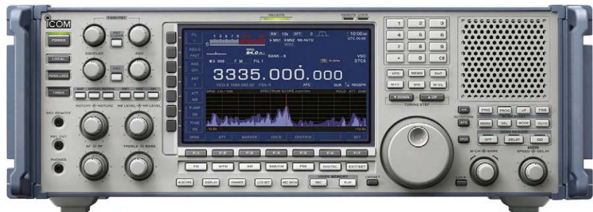
FIGURE 7.18 Icom R-9500 Has a Built In Video Decoder, Reprinted with Permission Icom America Inc. ©2012 Icom America Inc. The Icom Logo is a Registered Trademark of Icom Inc. The Use of Icom Product Images has been Approved for Tutorial Purposes
