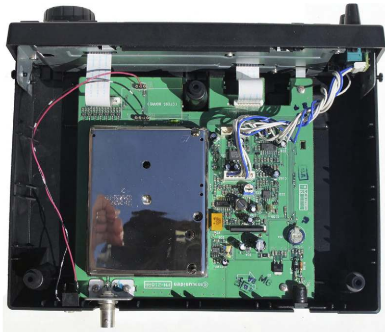
FIGURE 7.5 Scanner with a DIY Discriminator Out Added, Reprinted with Permission from Meagan Call
