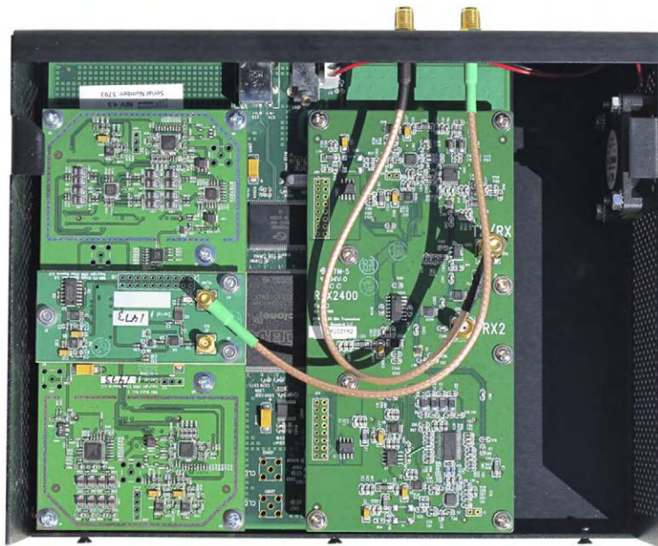
FIGURE 9.9 Inside of an Ettus USRP1 with the WBX and RFX2400 Daughter Cards Installed. Reprinted with Permission from Meagan Call
