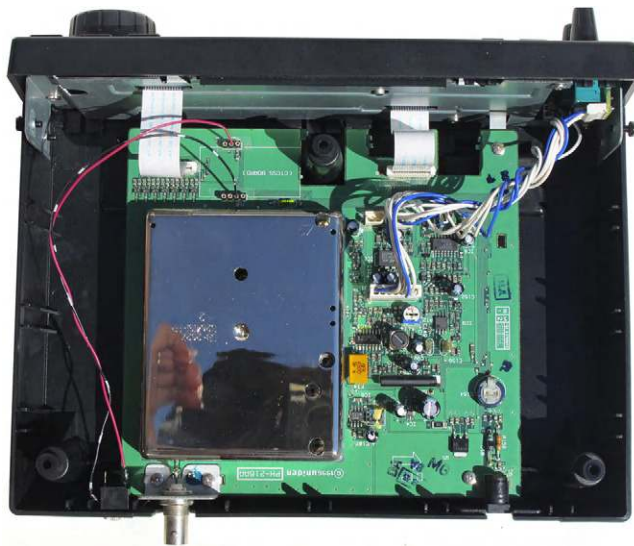
FIGURE 2.8 Inside of a Scanner with a DIY Discriminator Output Added, Reprinted with Permission from Meagan Call
