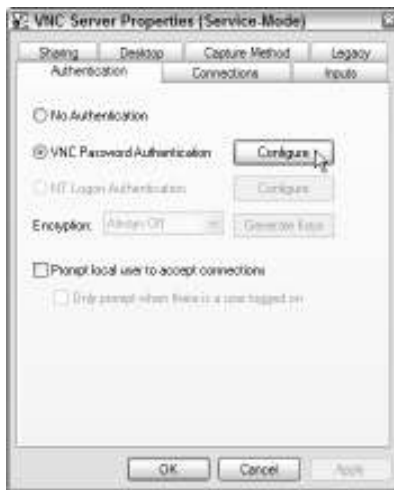
Figure 12-2: Here, you begin setting up a password for remote access.
