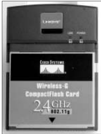
Figure 3-5: An example of a Compact Flash wireless adapter.
