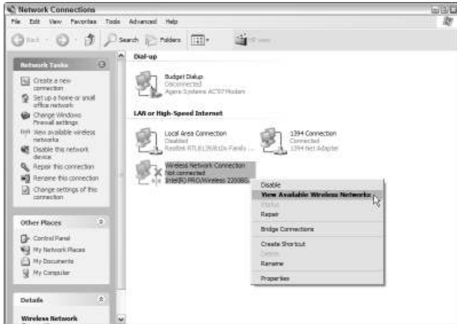
Figure 6-1: Launching the wireless zero con- figuration utility.
