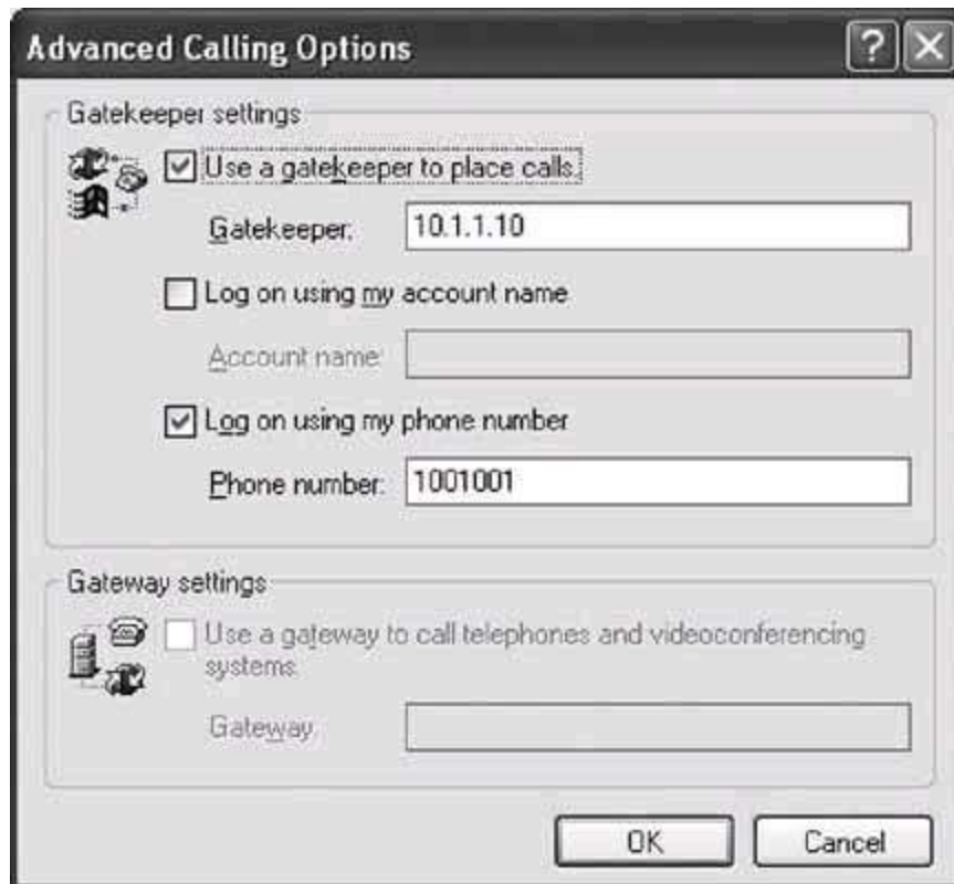
Figure 7-4. The NetMeeting Advanced Calling Options dialog box allows you to configure gatekeeper registration
