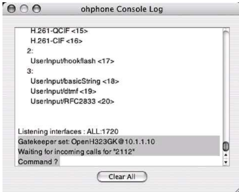
Figure 7-2. OhPhoneX's console log can help you troubleshoot the registration process
