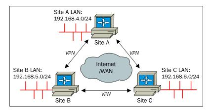
We will create three tunnels between the sites and set up redundant routes. That way, if one of the tunnels goes down, all the sites will remain visible to each other. However, this is at the cost of a performance penalty. Let's assume that the link between site A and site B goes down. The backup route goes from site A to site C to site B, so now traffic from site A to site B has to make an extra hop.
