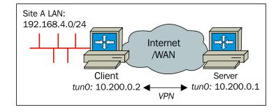
The client-side network **192.168.4.0/24** (with netmask 255.255.255.0) needs to be routed over the VPN tunnel to the server.
