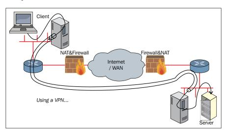
It should be noted that the preceding figure shows both the strengths and one of the greatest threats of VPN technologies. The VPN tunnel is *dug* through routers and firewalls on both sides. Thus, all the network traffic that is flowing via the VPN tunnel is bypassing the regular network defenses, unless special measures are taken to police the VPN traffic.
