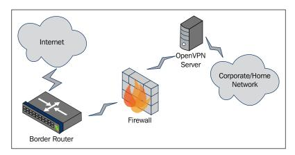
The next image shows how, logically, the firewall and the OpenVPN server can be on the same machine:
