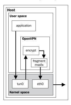
The flow of traffic from a user application via OpenVPN is depicted in the preceding diagram. In the diagram, the application is sending traffic to an address that is reachable via the OpenVPN tunnel. The steps are as follows:
