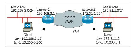
The public IP addresses used are not listed in this picture, but it is recommended to do so. Also, the connections from people working from home are not included, but they will connect to the public IP address of gateway1 in the preceding picture.
