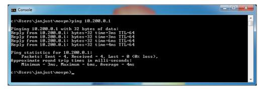
After we verify that we can reach the OpenVPN server, we need to ensure that the OpenVPN server is forwarding IP traffic and we need to add an extra route on the server side gateway to ensure that the VPN traffic is routed correctly back via the VPN server. Without this route, the machines on the server-side network will now know where the VPN traffic with IP addresses 10.200.0.0/24 is coming from, and will most likely wrongly route or drop the packets:
