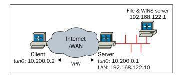
The server-side LAN is **192.168.122.0/24**, and on this subnet, the resources are located that the VPN clients need to access.
