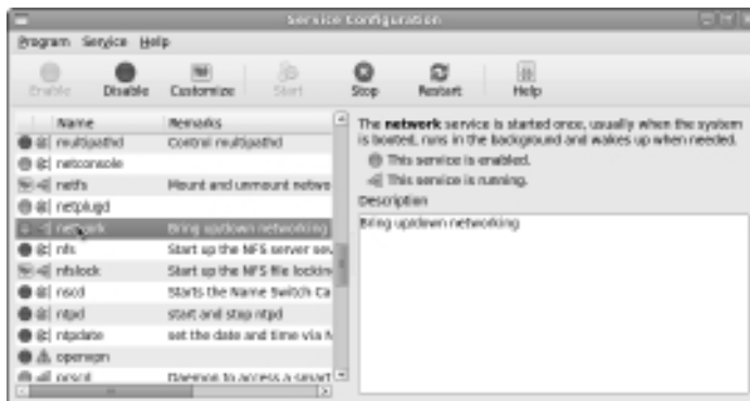
Figure 3-5: The Service Configuration window.
