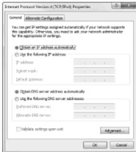
Figure 4-5: Configuring a Windows client to obtain its DNS address from DHCP.
