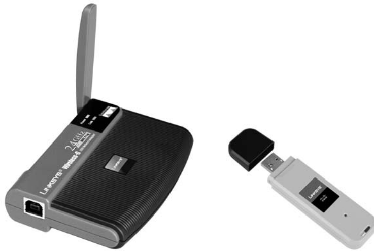
Figure 8-5: USB Wi-Fi adapters can be either stand-alone devices (left) or small plug-in modules (right).
