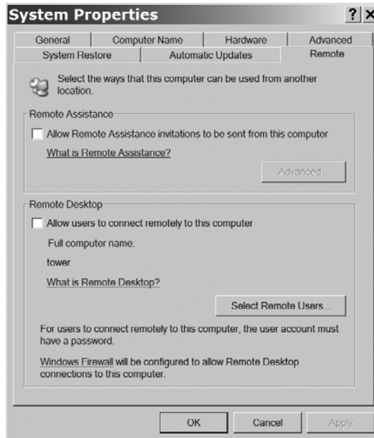
Figure 16-1: The Remote tab in System Properties controls inbound and outbound access to the Windows Remote Desktop utility.
