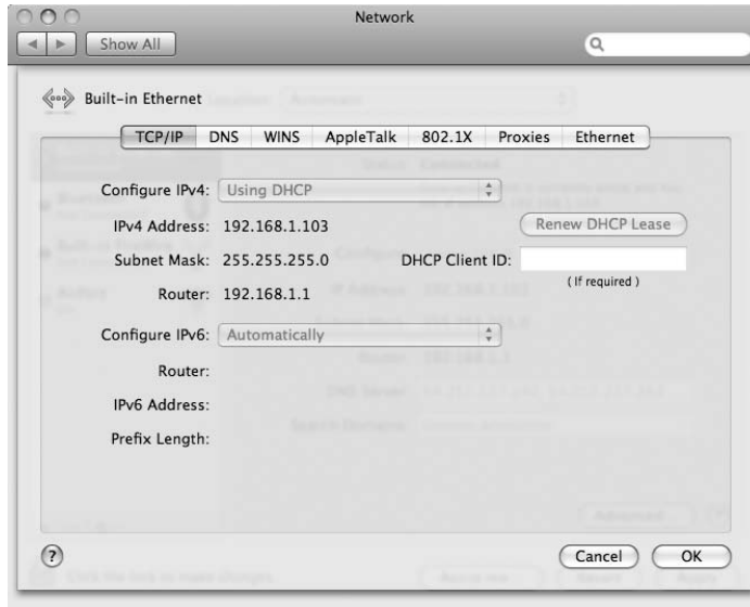
Figure 10-3: In OS X, choose the Using DHCP option to obtain an IP address from a server.
