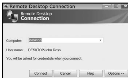
Figure 16-3: Use the Remote Desktop Connection dialog to specify the computer you want to control.
