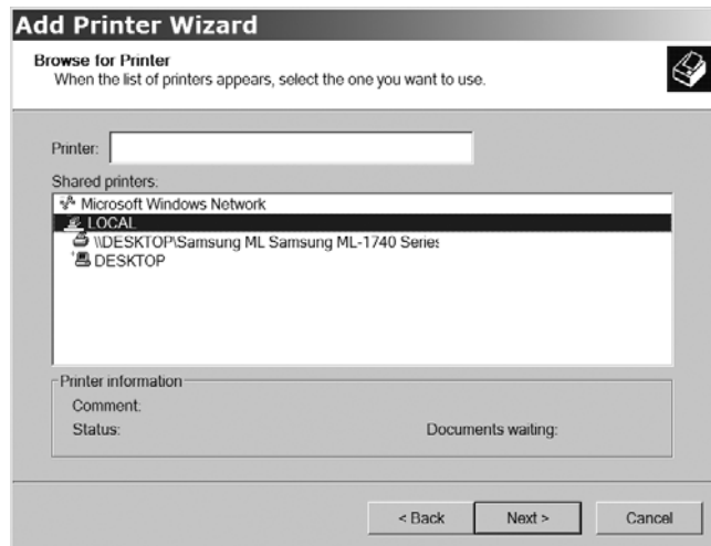
Figure 14-5: The Browse for Printer screen shows a list of all the shared printers connected to this network.
