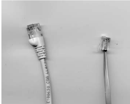
Figure 7-1: An RJ-45 data plug (left) has eight wires; an RJ-11 telephone plug (right) has four or six wires.
