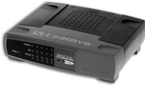
Figure 3-4: This switch connects five network nodes.
