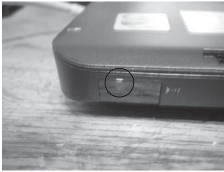
Figure 2-8: The IrDA port on a laptop computer often looks like a blank panel on the edge of the case.
