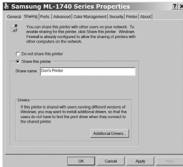
Figure 14-4: Use the Sharing tab of the printer's Properties dialog to turn on sharing.
