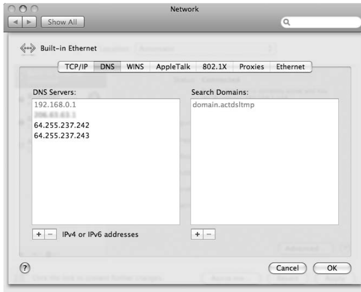
Figure 11-14: Enter the addresses of your ISP's DNS servers in the DNS window.
