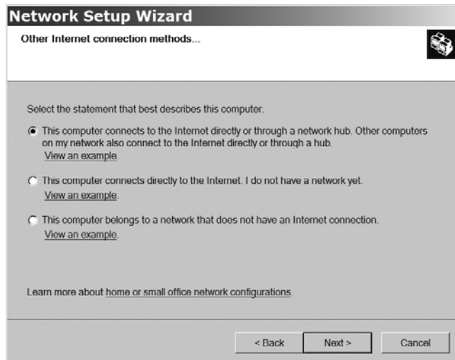
Figure 11-3: Select the This computer connects to the Internet directly or through a network hub option to connect to your LAN.
