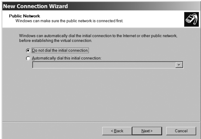
Figure 13-8: In a wireless network, the VPN does not require a dial-up connection.
