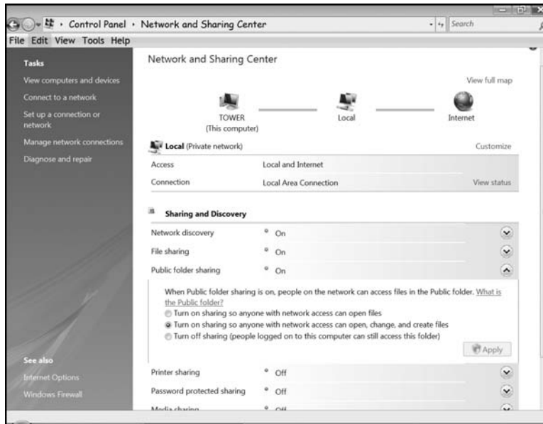
Figure 12-5: The Network and Sharing Center controls the access level for the Public folder.
