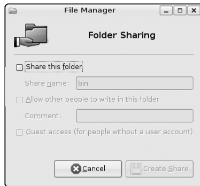
Figure 12-17: Use the Folder Sharing dialog to configure a directory as a network share.
