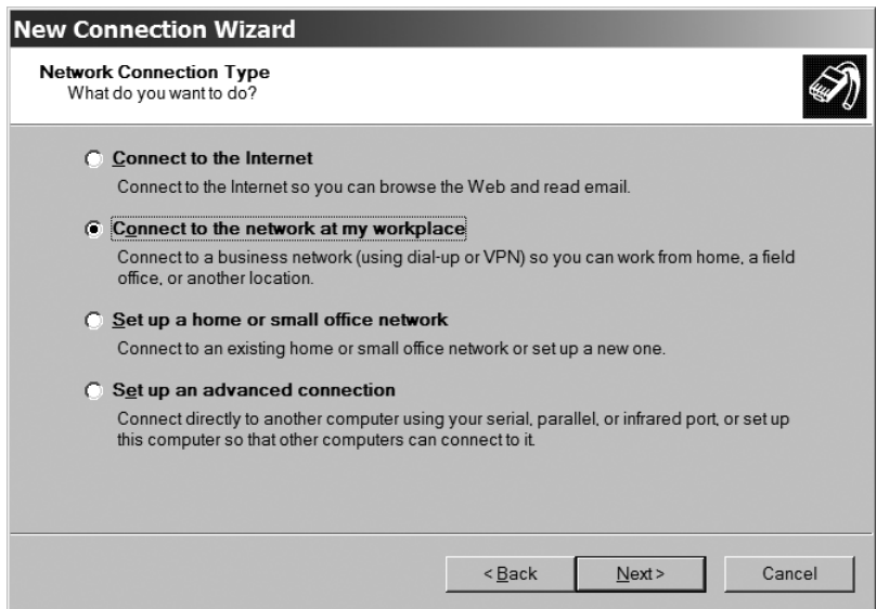
Figure 13-6: The option for creating a VPN link specifies connecting to a workplace network, but this option also applies to a wireless VPN.
