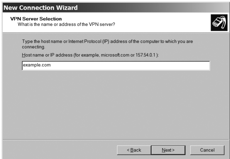
Figure 13-9: The host name or IP address identifies the VPN server at the other end of the wireless link.
