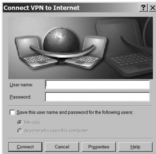
Figure 13-12: Use the Connect VPN to Internet window to configure a VPN in Windows XP.
