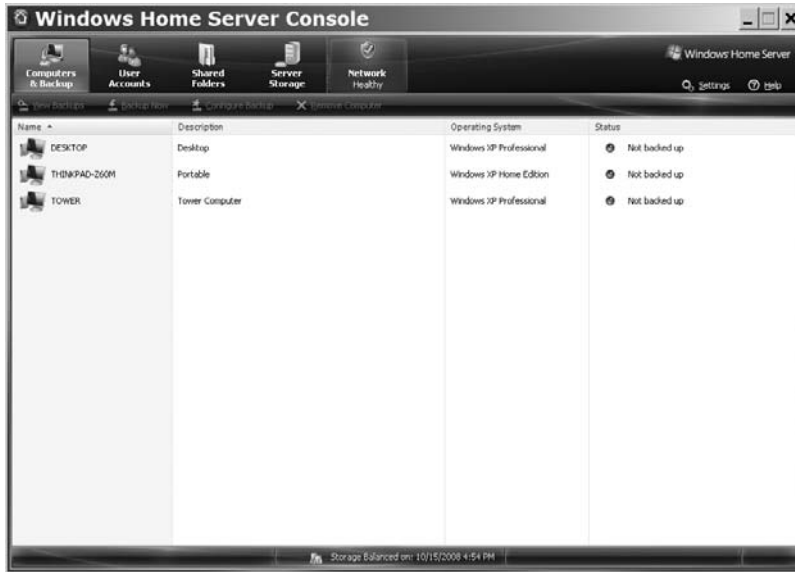
Figure 9-1: The Windows Home Server Console offers many control options on a single screen.
