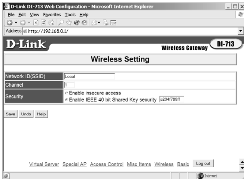
Figure 13-18: The configuration utility for a D-Link access point accepts WEP keys in hex format.
