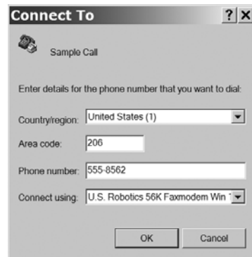
Figure 2-10: The Connect To dialog in HyperTerminal includes space for an area code and telephone number.
