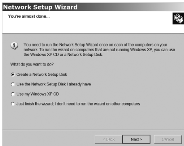
Figure 11-6: The Network Setup Wizard will offer to create a Network Setup Disk.
