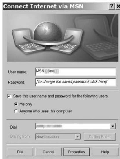
Figure 2-9: The Connect dialog in Windows specifies the telephone number that a modem will call and the login and password that the computer will send after the connection goes through.
