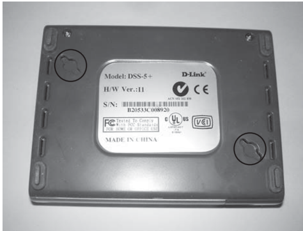
Figure 6-7: This D-Link switch has keyhole slots on the bottom of its case.
