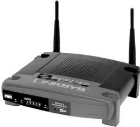
Figure 2-10 A wireless router combines an access point, a switch, and a router
