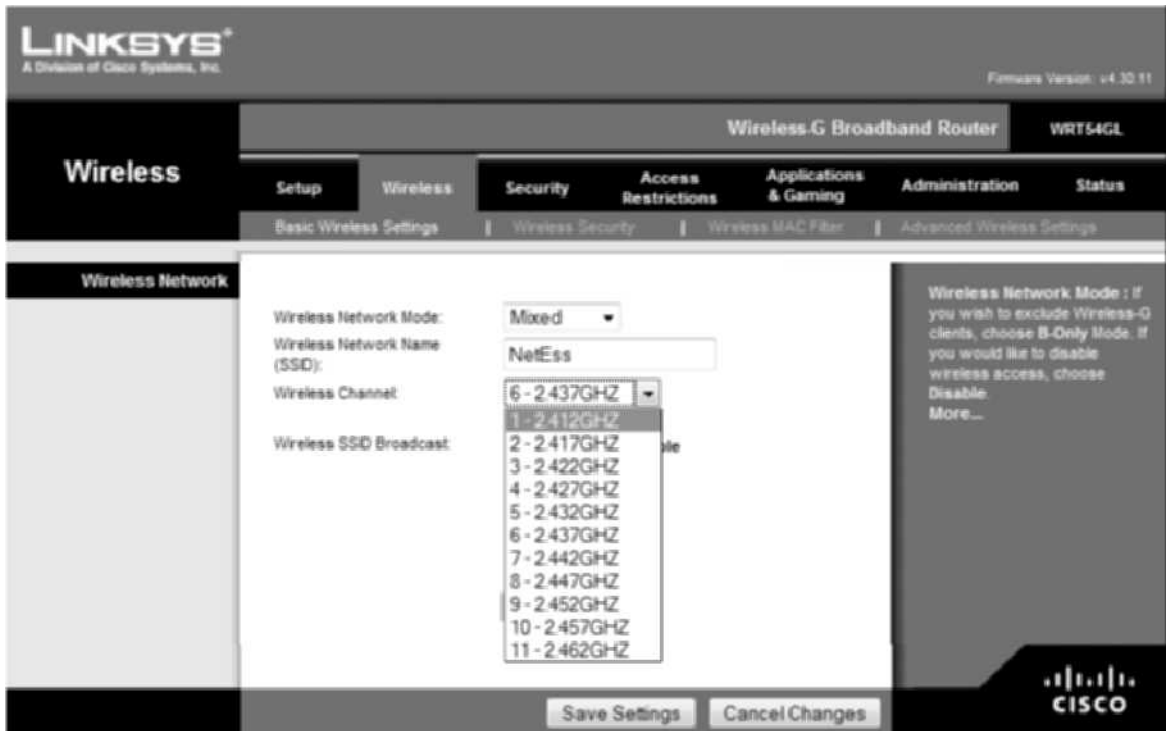
Figure 3-18 Selecting a Wi-Fi channel on an access point
