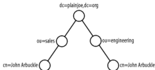
Figure 4-2. Using organizational unit to avoid collisions of common names (cn)
