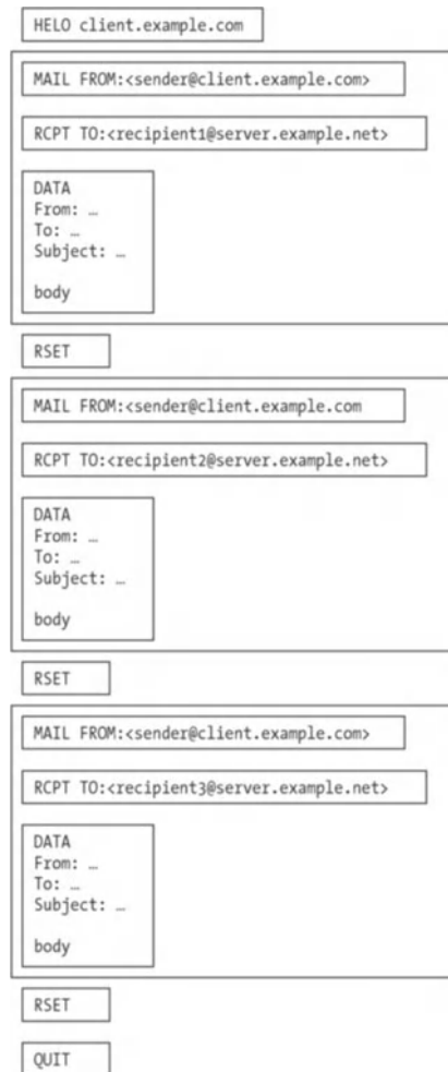
Figure 12-1. One SMTP connection, three messages
