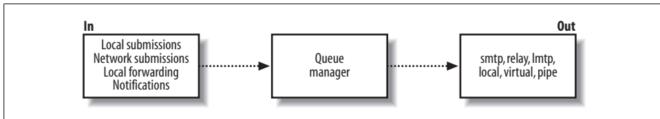
Figure 3-1. Broad view of the Postfix architecture
