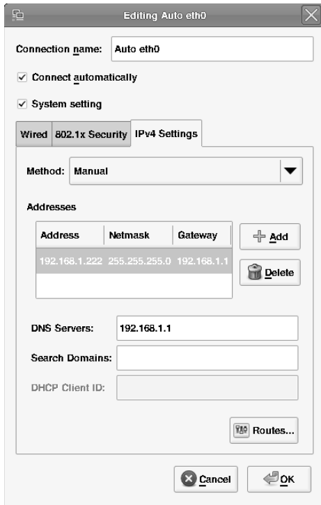
Figure 6-6: If you want to assign a static IP address to your client, you have more work to do.
