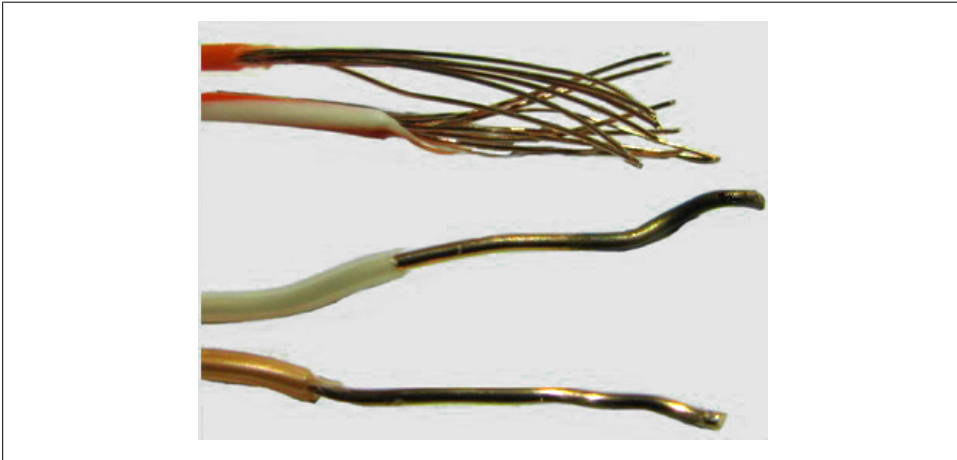
Figure 2-17. Stranded vs. solid core cable
