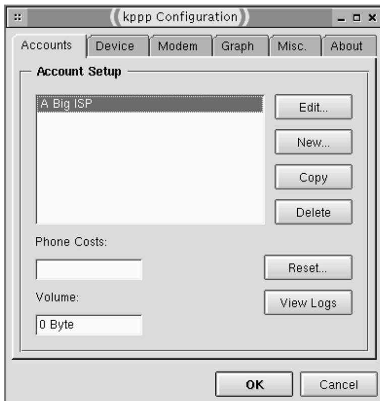
Figure 2.5. The KPPP Configuration dialog box controls hardware features associated with a PPP connection, such as what modem device to use, and lets you modify specific accounts using other dialog boxes.
