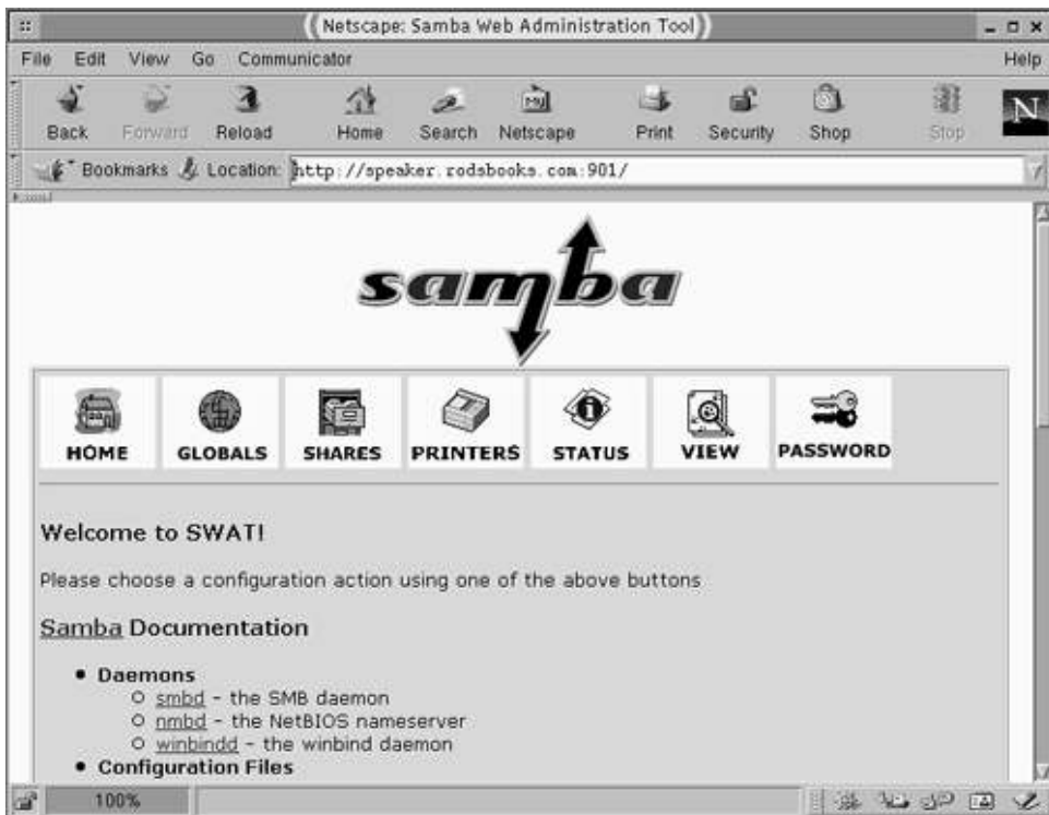
Figure 16.8. The main Samba configuration page allows you to select configuration areas or view Web based Samba documentation.
