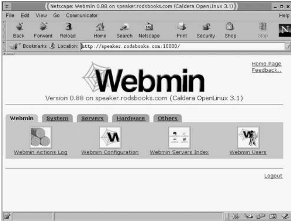
Figure 16.5. Webmin's main screen lets you select the general category and, when that's chosen, the specific subsystem you want to configure.
