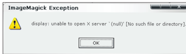
Fig 5-1: The Error Message when Windows is not Running an X Window Server such as Xwin32
