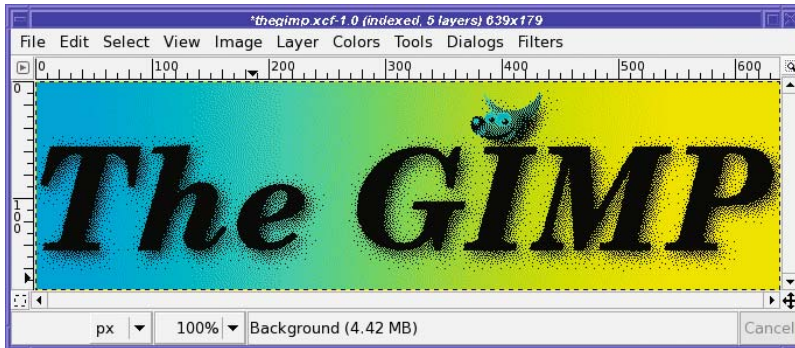
Figure 8-27. An 8-color palette with Floyd-Steinberg ( reduced color bleeding ) dithering and dithering of transparency
