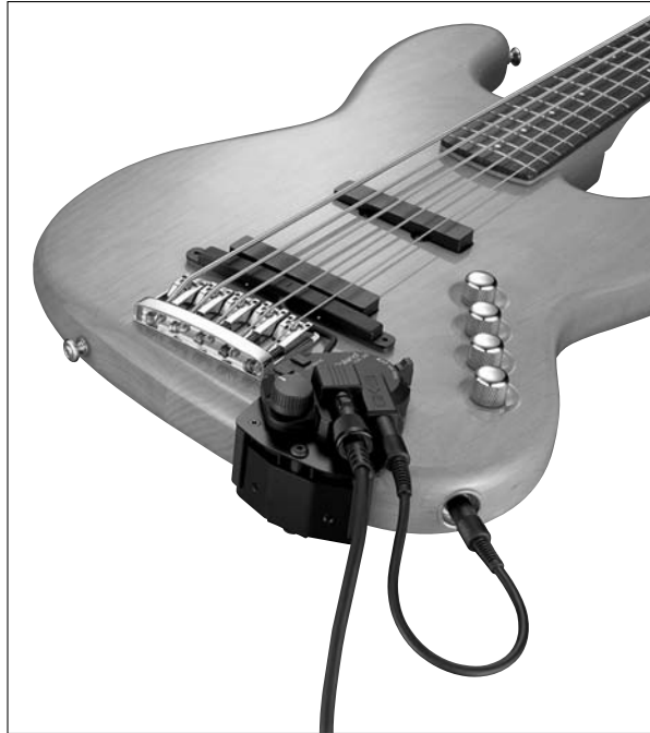
Figure 4-3: An electric bass with the Roland GK-3B Divided Pickup for Bass attached.
