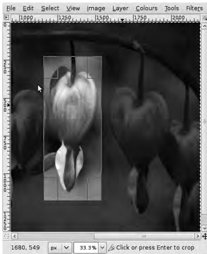
Figure 3-25. You can modify the Crop tool's selection by moving the corner rectangles or by dragging the selection edges.
