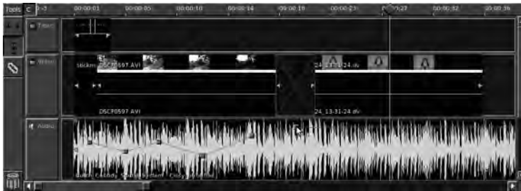
Figure 11-27. Open Movie Editor's audio volume automation works in a similar way to the Ardour editor's level automation.
