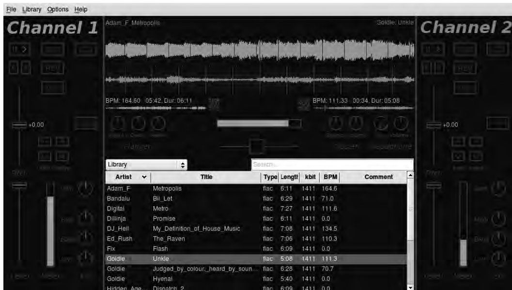
Figure 8-12. Wideboy, a custom Mixxx skin I adapted from outlineSmall for the Indamixx tablet computer. Note the unusual aspect ratio; the dimensions of the skin background are 1024 x 575 pixels.
