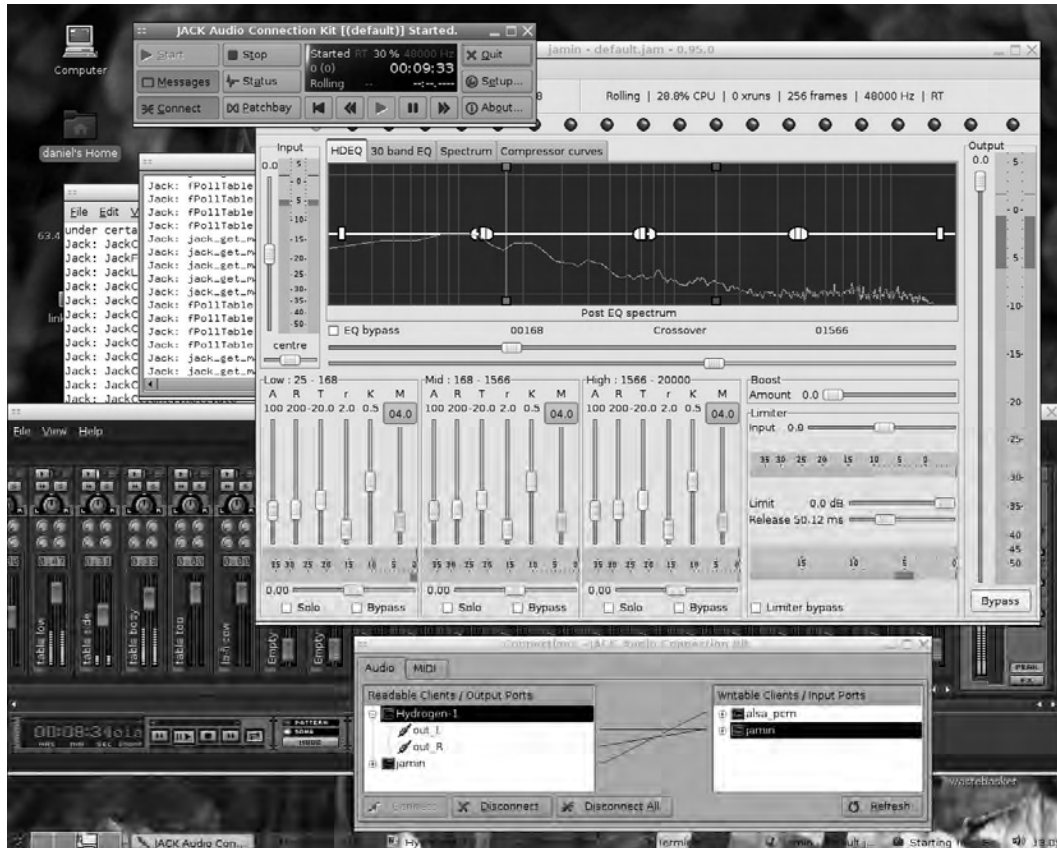
Figure 1-7. The 64 Studio desktop, showing the JACK sound server and JACK client programs Hydrogen and Jamin
