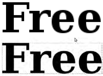
Figure 4-1. You can scale vector graphics to any size without losing quality, making them an excellent format for original artwork and typography. Above, a pixmap of a 48-point font scaled to 400%—below, the same font drawn as a vector, scaled to the same size.
