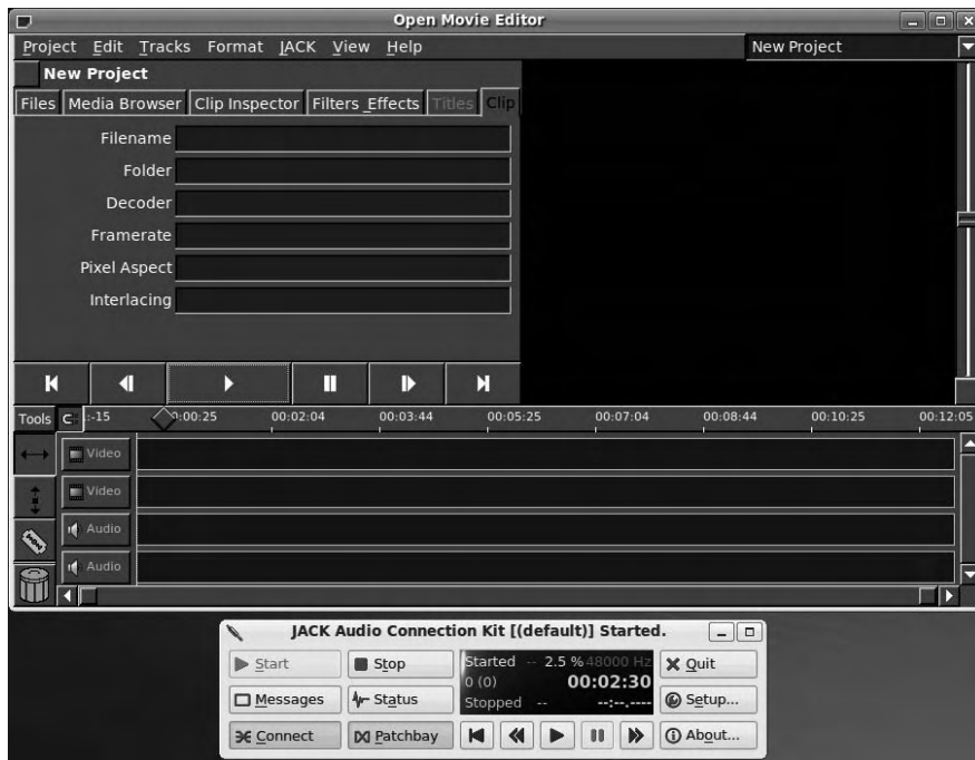
Figure 11-18. Start JACK, and then run Open Movie Editor and resize its interface so that you can see all the tabs on the left side of the main window.
