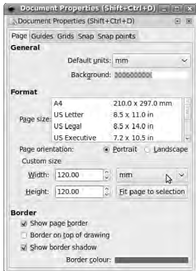
Figure 10-27. Set the Inkscape document size to ensure correct alignment in the printer.
