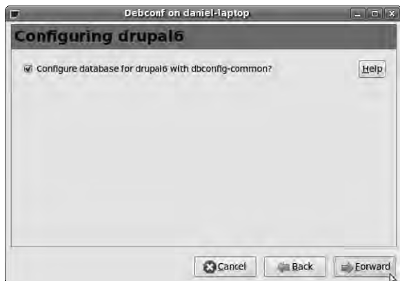
Figure 12-7. Let debconf run the database configuration tool for Drupal automatically, unless you know that you shouldn't.
