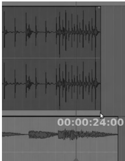
Figure 9-42. Use the mouse in Object mode to trim region start and end points.
