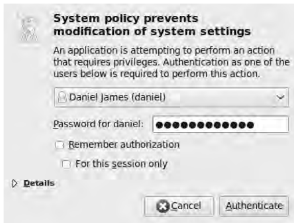
Figure 2-32. All software installed system-wide on Ubuntu requires your password, entered here into a dialog box. Don't check the "Remember authorization" box if anyone else has access to your computer; if you do, the password check is bypassed.
