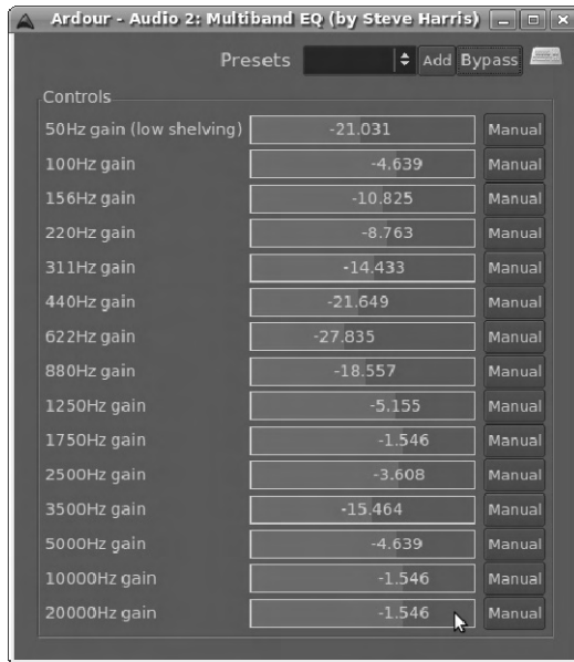
Figure 10-9. This multiband EQ with a low shelf enables you to shape the frequency curve of your track.
