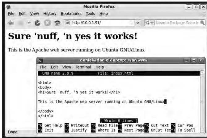
Figure 12-5. Editing Apache's default web page shows that the web server is really running.
