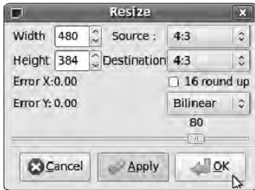
Figure 11-11. Adjust the output frame pixel dimensions with the MPlayer resize filter. If you can't get the correct numbers, you may need to go back to the cropping stage.
