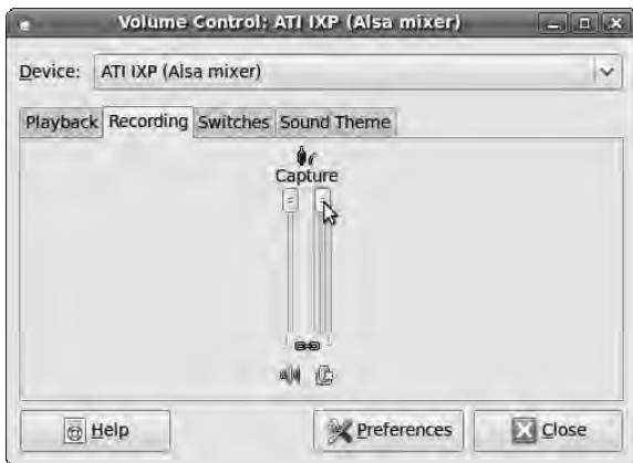
Figure 9-8. You probably need to adjust the system's input-level controls and capture switches.
