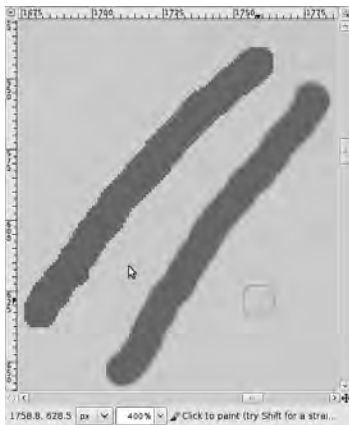
Figure 3-36. Zoomed in to 400% of normal size, the difference in edge between the Pencil tool (left) and the Paintbrush tool (right) is obvious.
