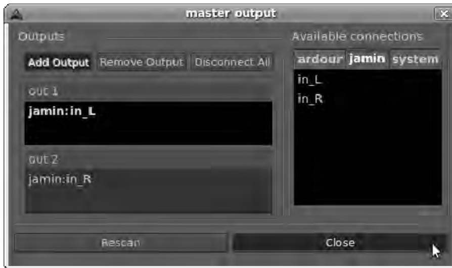
Figure 10-11. JAMin connected between Ardour’s master bus outputs and the first two ports of the internal soundcard
