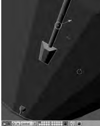
Figure 6-33. After duplication, join the opposite pair of lug and rod models into a single object so that they can be duplicated again.
