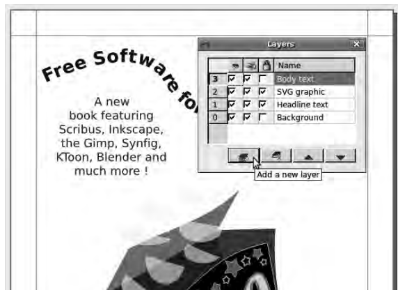
Figure 7-32. Using layers in Scribus helps to isolate different parts of a layout, which can be locked into position.
