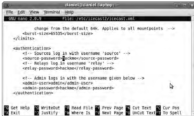
Figure 12-40. The Icecast package is distributed with default passwords and not very good ones either.
