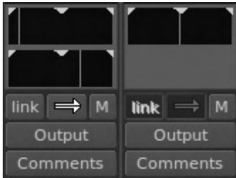
Figure 10-5. Stereo track on the left, featuring two-channel panning. Mono track on the right, panned to center.
