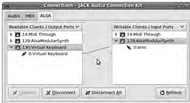
Figure 8-35. You can use the JACK Control applet to make a MIDI connection from Virtual Keyboard to AlsaModularSynth.
