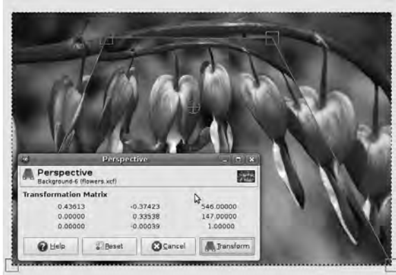
Figure 3-29. You can fake perspective effects using the tool of the same name. The center of the effect is adjustable using the blue crosshairs.
