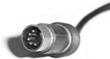
Figure 8-26. The obsolete five-pin DIN plug is still used for MIDI data. Photo by Boffy B, public domain.
