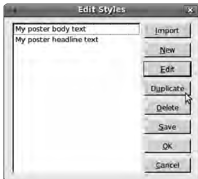
Figure 7-16. The small Edit Styles dialog allows style sheets to be duplicated, edited, and deleted. A headline style has been created, based on the previously defined body text style.
