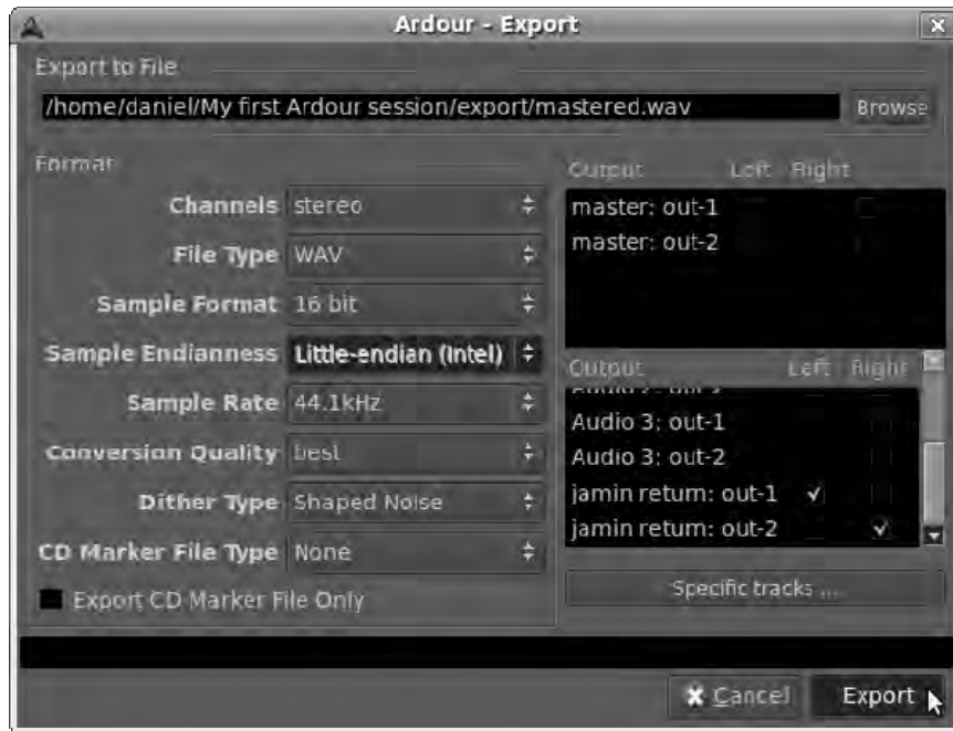
Figure 10-19. Make sure you check the correct output boxes when exporting from the jamin return bus.
