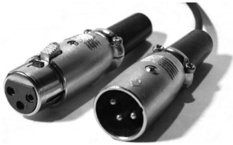
Figure 9-3. Decent analog microphones standardized on the three-pin XLR connector, shown here in female and male variants, many years ago. Some newer microphones connect via USB instead. Photo by Michael Piotrowski, GNU FDL.
