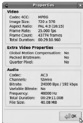
Figure 11-8. The Properties dialog provides details about the resolution and codecs of the source video.
