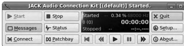
Figure 8-30. JACK Control displays the load on the system and the current sample rate.
