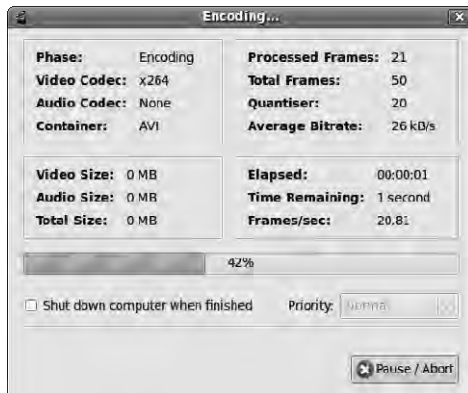
Figure 11-3. The progress bar indicates how long you have to wait for your video to be encoded. If it's a long video and your computer is slow, it may be time to order a pizza. This simple example has only 50 frames of animation, which are being encoded at around 20 frames per second.
