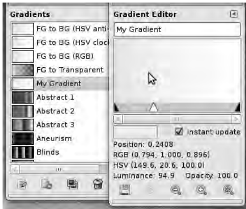
Figure 3-35. Right-click in the Gradient Editor's preview window to set the left and right colors.
