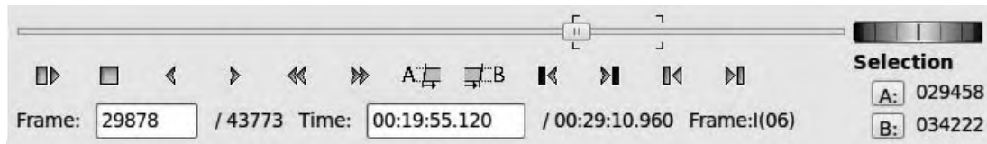
Figure 11-13. The selection points set with the A and B transport buttons are shown as square brackets on the timeline.
