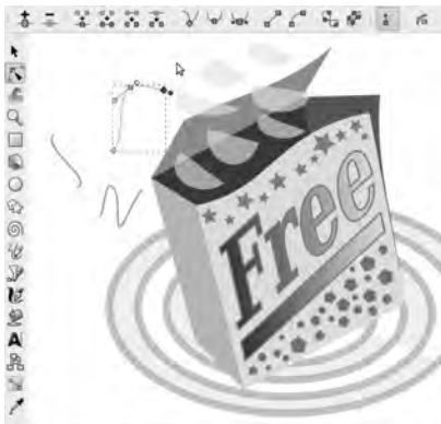
Figure 4-16. The Draw Freehand Lines tool creates Bezier curves, with width, color, and style set by the active Stroke properties. Switch to the Edit Paths tool, and the lines are ready to be modified.
