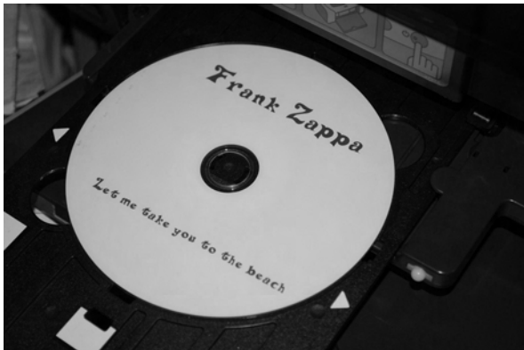
Figure 10-26. Epson's ink-jet printers can print on the CD surface, if you're prepared to coax them a little.
