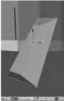
Figure 6-31. Model the drum lug by selecting and moving or scaling control points to create an irregular shape.
