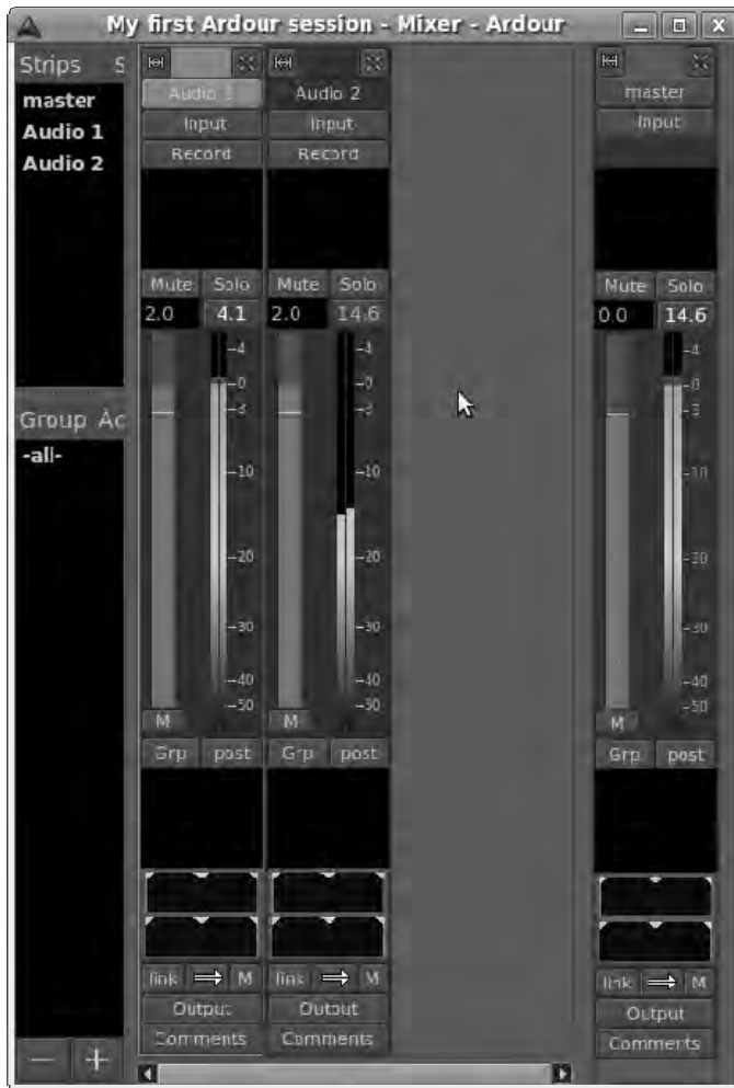
Figure 10-4. You're running way too hot here—a session mixed like this will sound pretty rough on CD.
