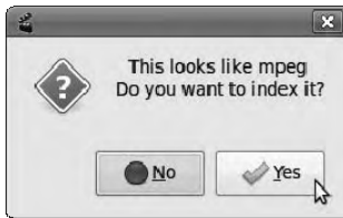
Figure 11-4. MPEG data imported from DVD VOB files must be indexed before it can be edited in Avidemux.
