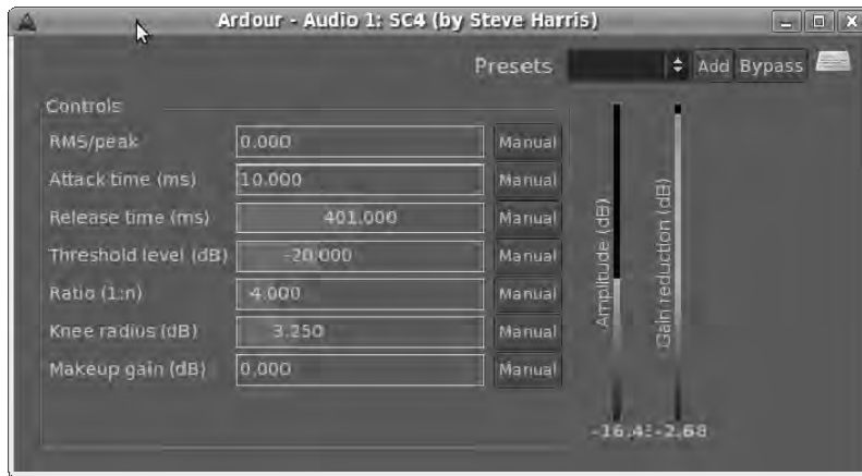
Figure 10-7. Some typical settings for the SC4 compressor. The “Gain reduction” meter shows a -2.68dB cut on the Audio 1 track, but this value varies continuously according to the input amplitude.
