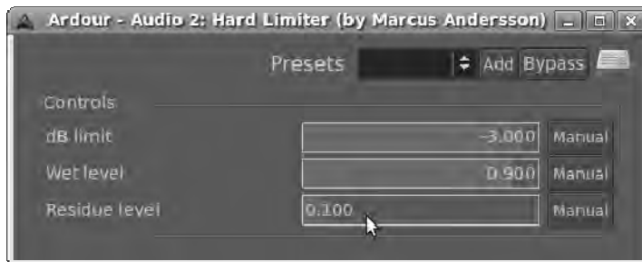
Figure 10-8. You can use the Hard Limiter plug-in to prevent transients from causing overs.
