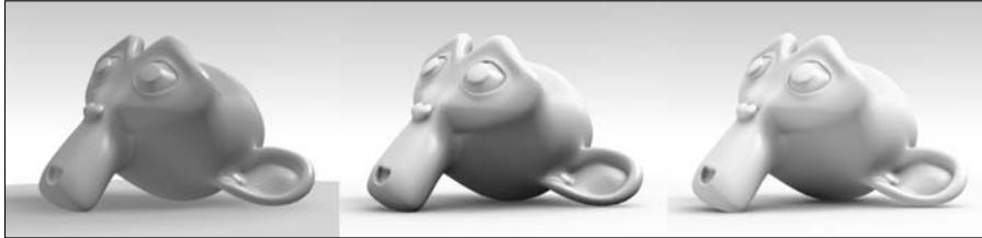
Figure 9-17: From left to right, with their render times: no AO, raytraced AO, and approximate AO.
