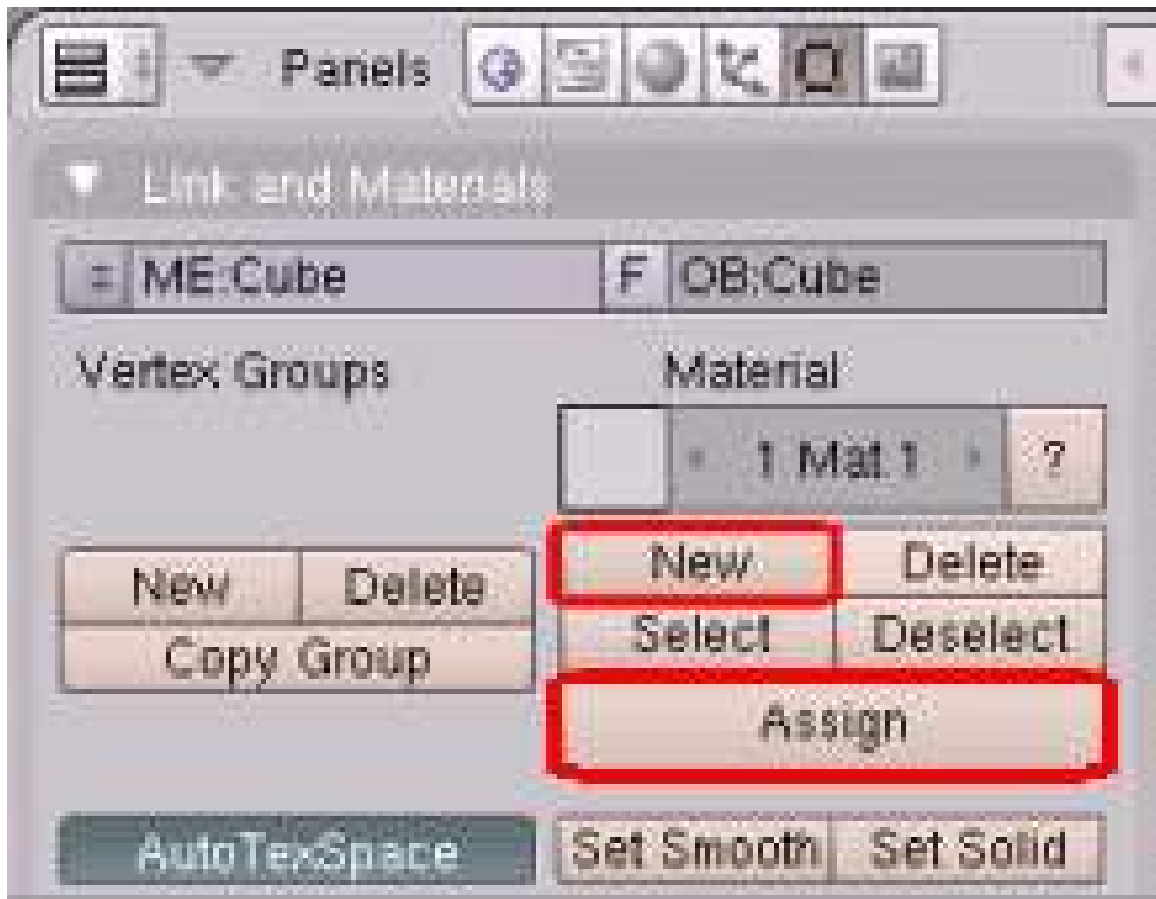
Figure 884 Press the 'new' button then the 'assign' button to assign a material to a number of faces
