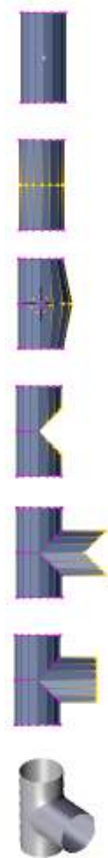
Figure 520 Figure 1: Modeling a simple T joint.
