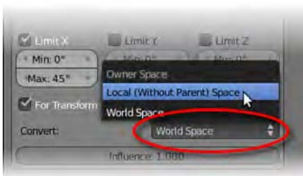
Figure 7–20. The Limit Rotation constraint has the option to use local space.
