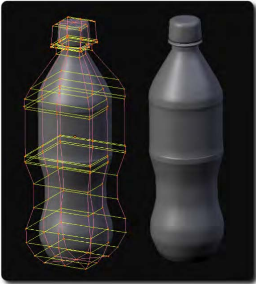
Figure 6-33. This NURBS version of the bottle is smoother than the polygon spin version made earlier, and it contains about a third of the points.
