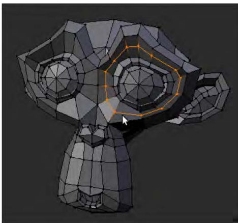
Figure 3–13. Adding a new edgeloop
