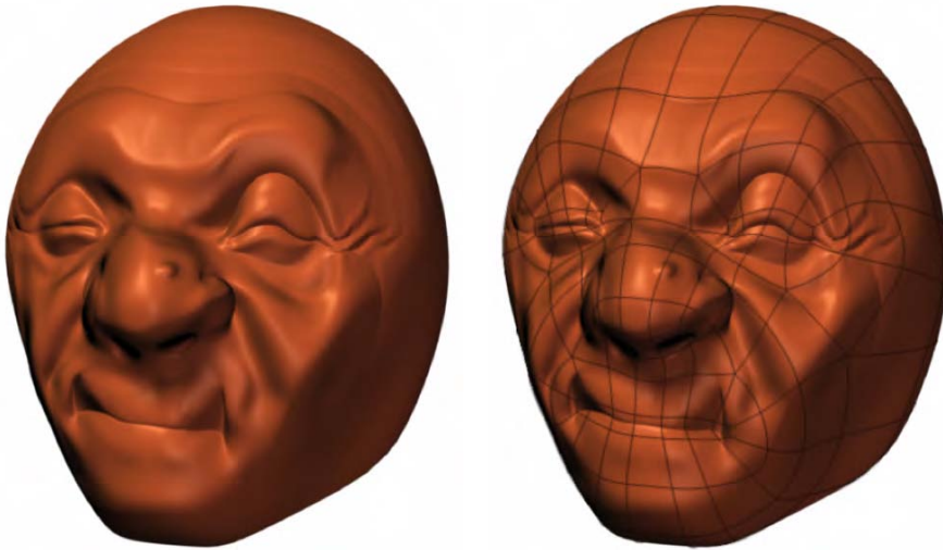
Figure 5–34. The final result (left) looks highly detailed, but the mesh is actually low resolution (right, showing wire).
