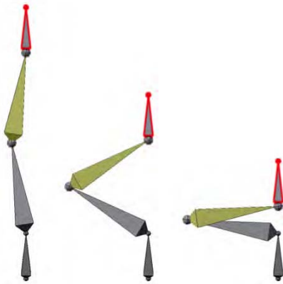
Figure 8–5. Once set up, an IK constraint causes the arm to bend when the hand (shown in red) is moved.
