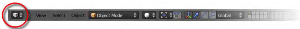
Figure 2–6. Header strip with the window type set to 3D View (cube icon)
