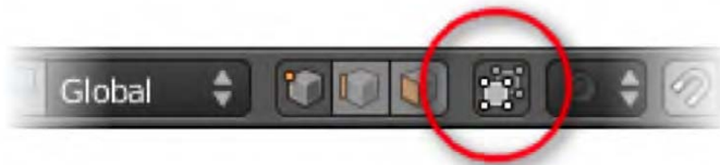
Figure 3–9. The occlusion button (aka “Limit selection to visible”)
