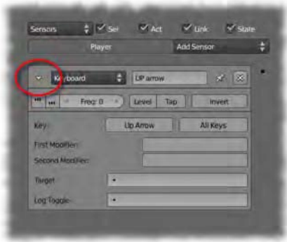
Figure 11–13. Completed “Up arrow” sensor with minimize button circled
