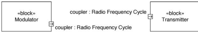
Figure 3.13 Blocks with atomic flow ports
