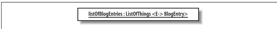
Figure 6-12. The listOfBlogEntries reuses the generic ListOfThings template, binding the E parameter to the BlogEntry class to store only objects of the BlogEntry class
