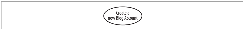
Figure 2-5. A use case in UML is drawn as an oval with a name that describes the interaction that it represents
