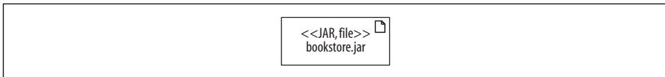
Figure B-3. The bookstore.jar has both the JAR and file stereotype applied to it
