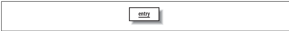
Figure 6-2. You show an instantiated object by using a rectangle but with the name of the object—its identifier—underlined
