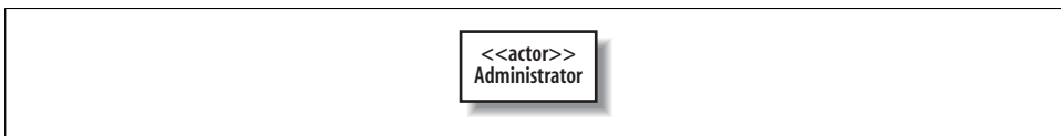
Figure 1-11. The Administrator element is still an actor, but its stereotype is now specified using a name rather than an icon
