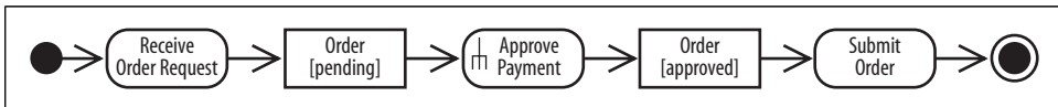
Figure 3-18. The focus of this diagram is the change of state of the Order object throughout the order approval process
