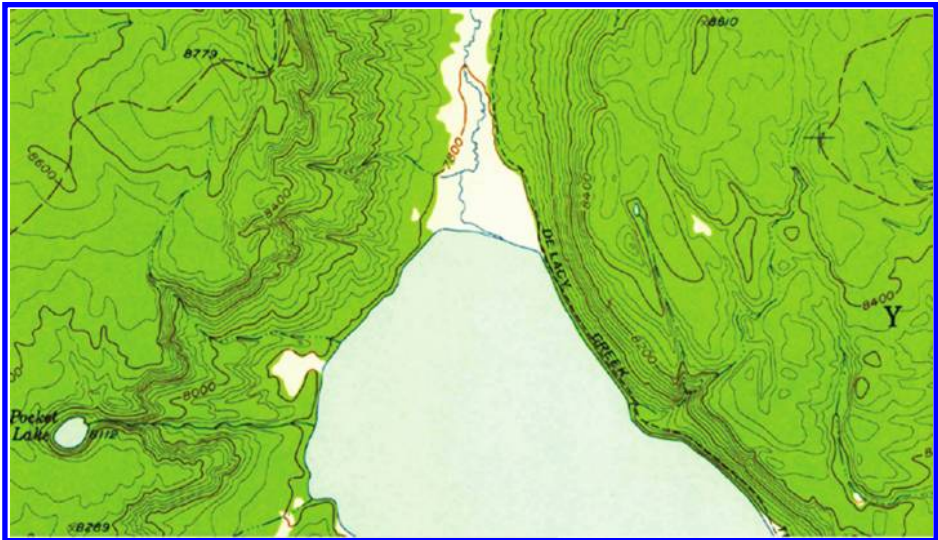
Figure 6.13 This image shows a sample of a professionally made map with contours. Closely spaced contours reflect steep slopes. Source: USGS, The National Map, US Topo , http://nationalmap.gov/ustopo/index.html
