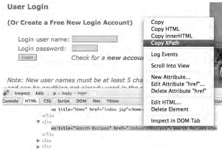
Figure 10-2. Using Firebug to copy the XPath to any HTML element on a web page
