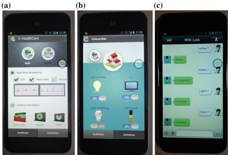
Fig. 10 Screenshot of smart phone used by the wheelchair user. a The smart phone perceives the vital physiology parameter of wheelchair user. b The smart phone controls the local shared household equipment via remote online resource. c A wheelchair user interacts with RFID lock via WeiChat, a IM of online social network
