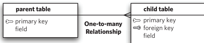
Figure 7.1 A basic data model. The white key icon indicates a primary key, and the gray key icon indicates a foreign key.
