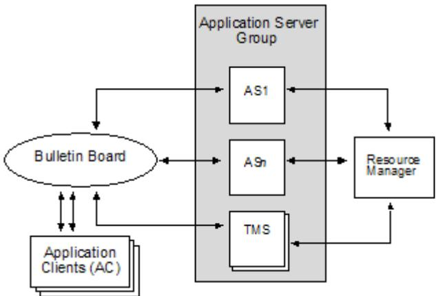
Multiple application client programs communicate with multiple application servers that are combined into *server groups*. Messages are routed between clients and servers through the Tuxedo bulletin board. Transaction manager servers in each server group manage two phase commit protocol and recovery of global transactions.
