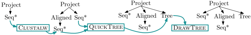
Fig. 6. Abstract flowgraph for Example 3 showing that QUICKTREE also uses the unaligned set of sequences as input and not just the aligned ones as was desired
