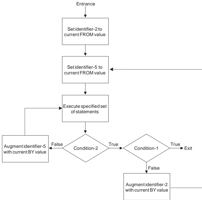
Figure 15. Varying Two Identifiers—with TEST AFTER
