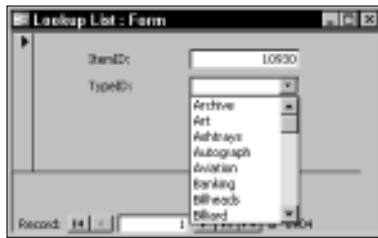
Figure 17-1: The TypeID field on this form is a lookup list that's in a combo box.
