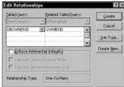
Figure 5-9: Use the Edit Relationships dialog box to specify the parameters for the relationship.
