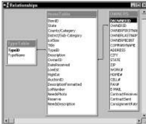
Figure 5-7: The Relationships window enables you to view, create, or edit table relationships.
