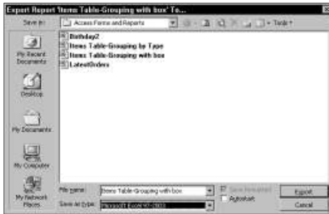
Figure 18-4: Use the Export Report dialog box to export a report in Excel format.
