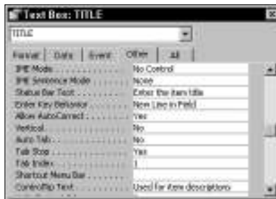
Figure 17-19: Use the Other tab of the Properties dialog box to add text prompts.
