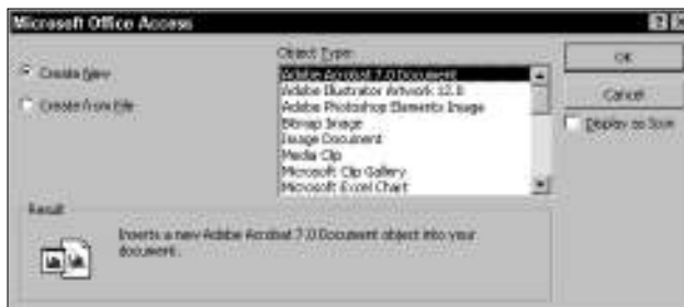
Figure 18-7: Use this dialog box to add new OLE objects to your database.
