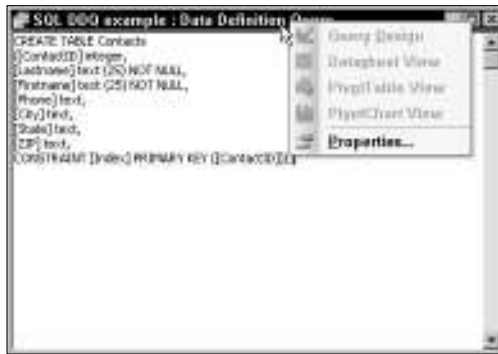
Figure 7-6: The pop-up menu has the Query Design option disabled for this query.
