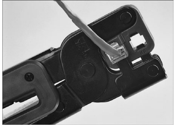
Figure 17.13 Firmly squeeze the crimping tool to attach the connector to the cable.
