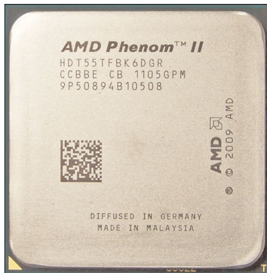
Figure 3.39 The Phenom II X6 conceals six cores and memory controllers for both DDR2 and DDR3 memory beneath its protective metal spreader plate.
