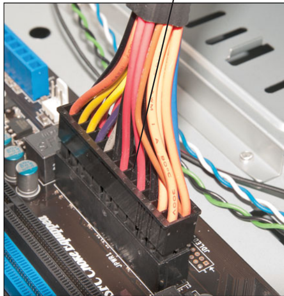
Figure 19.24 Attaching a 24-pin ATX motherboard power connector.
