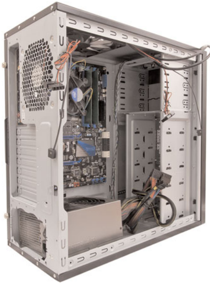
Figure 19.22 Installing the power supply into the chassis.
