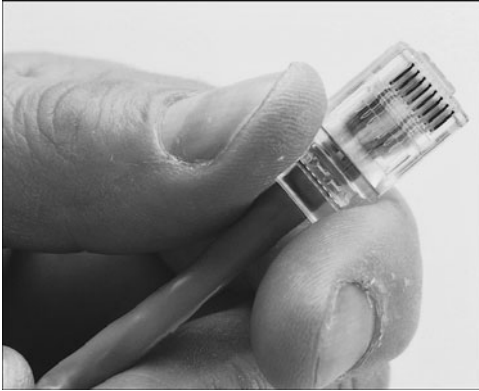
Figure 17.12 Push the 8P8C (RJ-45) connector into place, ensuring the cable pairs are ordered properly.
