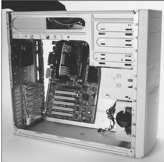
Figure 19.19 Installing a motherboard and tray into the chassis.
