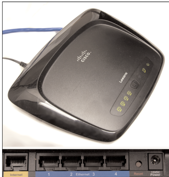
Figure 16.7 Front (top) and rear (bottom) views of a typical wireless router with a built-in four-port switch, the Cisco-Linksys Wireless-G Router, WRT54G2 v1.
