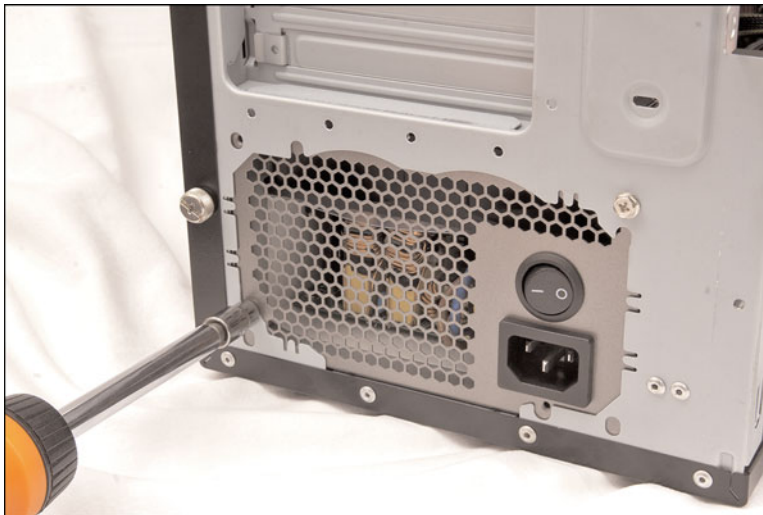
Figure 19.23 Installing the screws to retain the power supply.
