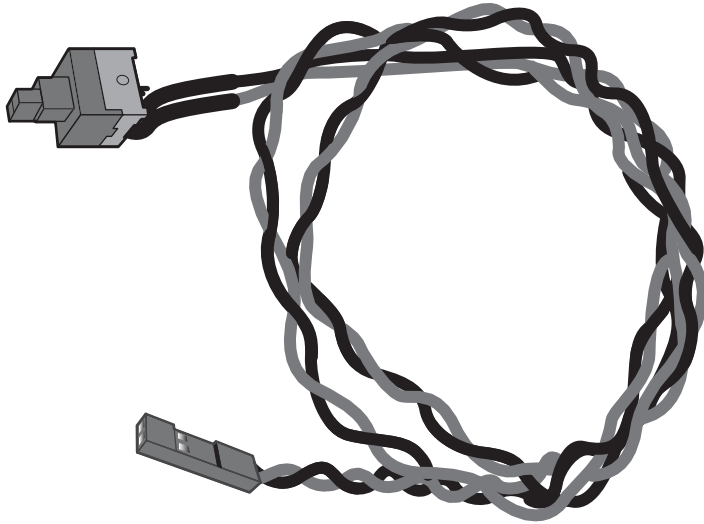
Figure 18.16 ATX power switch.
