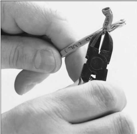
Figure 17.10 Carefully strip the cable jacket away to expose the four wire pairs.
