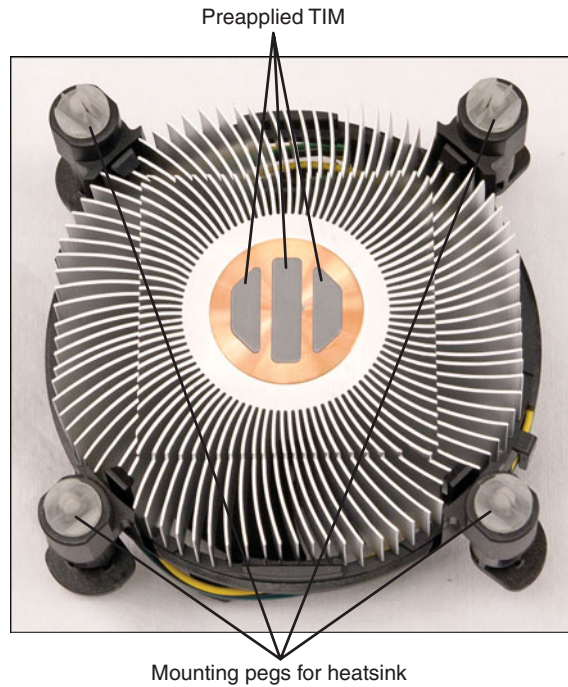
Figure 19.9 An Intel heatsink with preapplied TIM.
