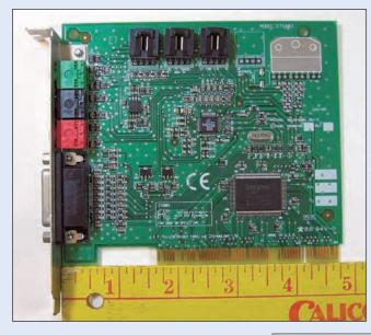
**Color Plate 14:** A PCI card. A PCI card's tabs are about 1<sup>5</sup>/<sub>8</sub> inches from the card's end.
