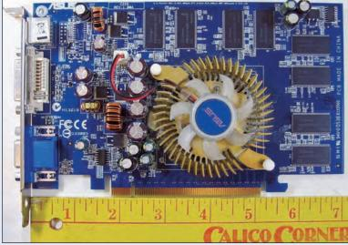
**Color Plate 16:** A PCI Express card. A PCI Express card's tabs are about 1<sup>3</sup>/4 from the card's end. Like AGP cards, most PCI Express cards have a little notched hook on the end that locks into the slot's plastic holder.
