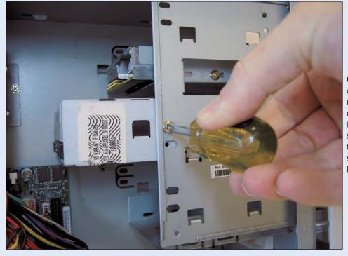
**Color Plate 27:** When cases don't include drive rails, you screw the drive directly to the case itself. (The screws are a slightly smaller size than the ones that hold cards in their slots, shown in Color Plate 19.)
