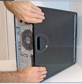
**Color Plate 3:** After removing the thumbscrews, slide the cover off by pulling it to the rear.
