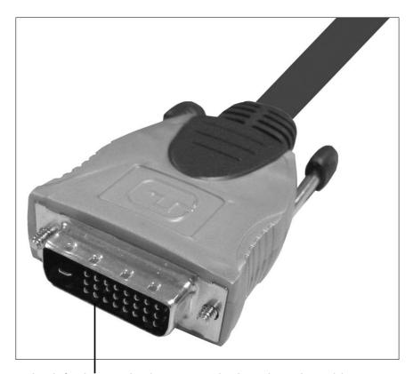
Check for bent or broken pins at both ends or the coble.
