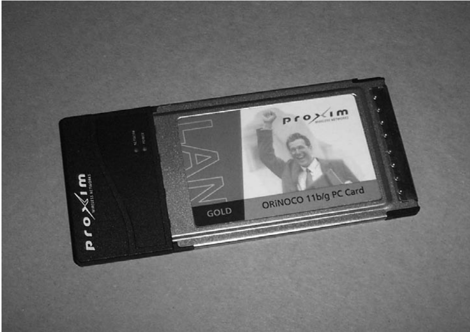
Figure 2.6 Proxim ORiNOCO 802.11b/g Wireless Card, front
