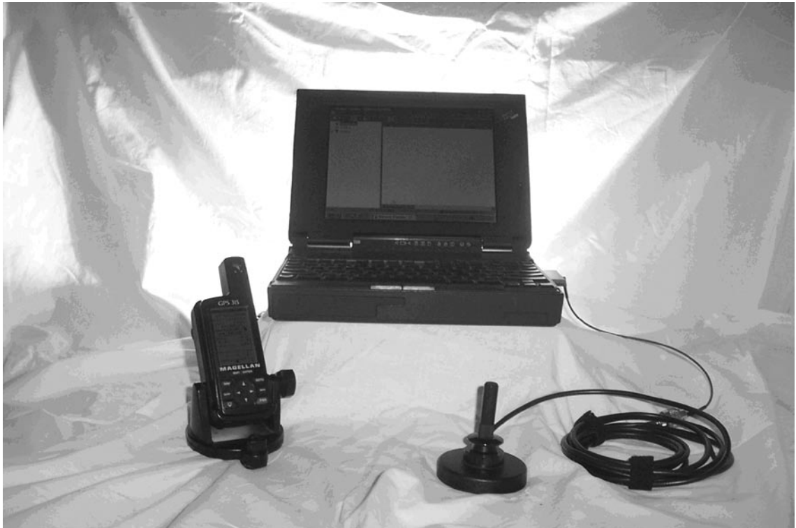
Figure 3.7 A Complete Kismet War Driving Rig; Laptop, GPS Receiver, Omni Antenna, and Pigtail
