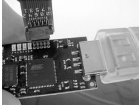
Figure 13-2 JTAG Programmer inserted into the RZUSBSTICK
