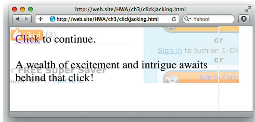
Figure 3.6 The overlay for a clickjacking attack
