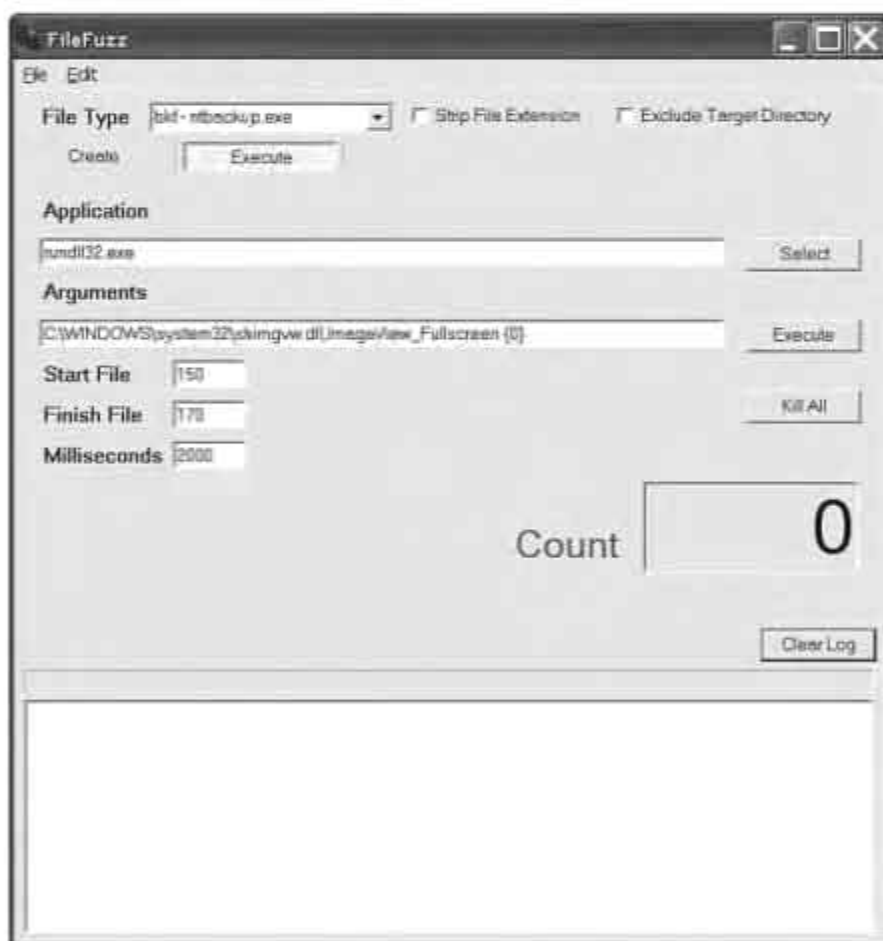
Figure 13.6 FileFuzz Execute tab settings for JPEG fuzzing
