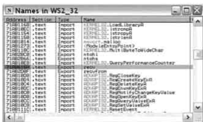
Figure 20.8 OllyDbg breakpoint on WS2_32.recv()
