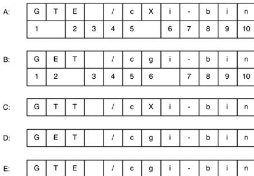
Figure 6-1. Desynchronization along packet boundaries with a GET request.
