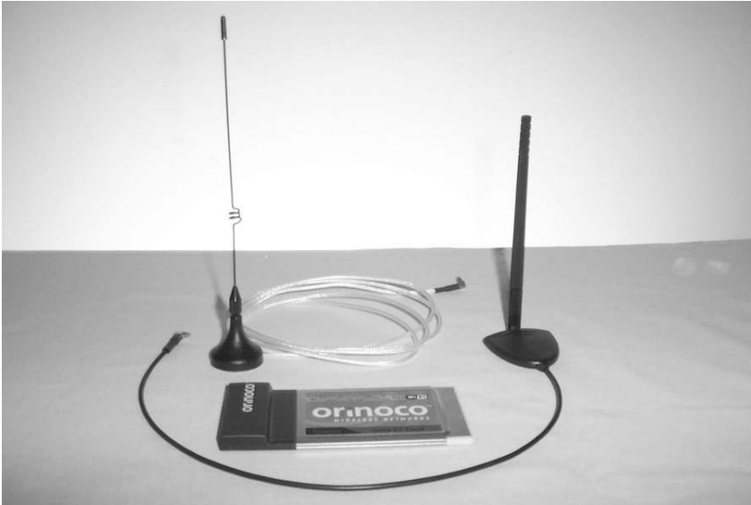
Figure 2.5 Small Omnidirectional Antennas - 5 dBi Gain
