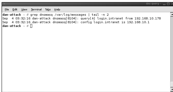
Figure 9.22 Client DNS Request with Reply to the IP Address of Your Web Server
