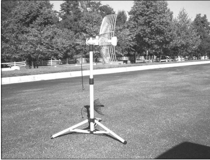
Figure 1.6 Parabolic Antenna Isn't Good for WarDriving
