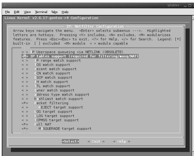
Figure 9.9 Enabling Iptables Support in the Kernel
