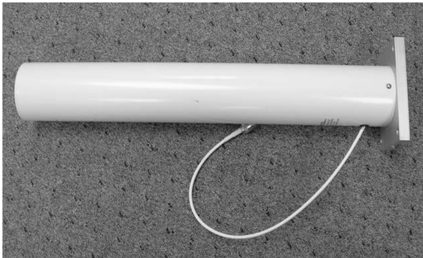
Figure 11.10 Directional Antenna (Hyperlink 14.5 Decibel (dbi))
