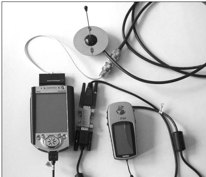
Figure 1.2 Typical PDA WarDriving Setup
