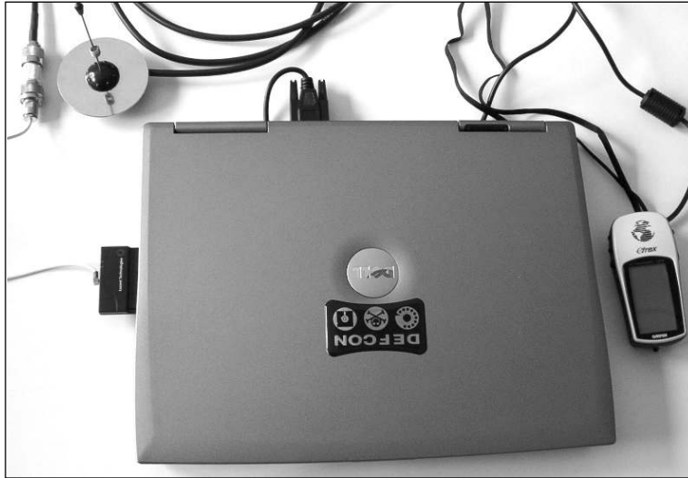
Figure 1.1 Typical Laptop Computer WarDriving Setup
