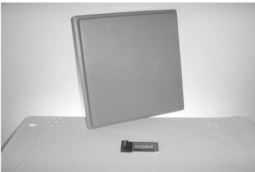
Figure 2.11 A Panel-type Directional Antenna; Shown with a Wireless Card for Size Comparison
