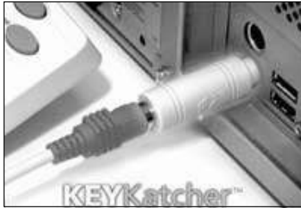
Figure 9.1 KeyKatcher with PS/2 Connectors
