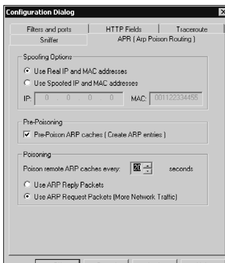
Figure 3.13 Cain Will Perform ARP Poisoning with a Single Click
