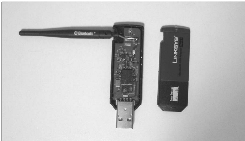
Figure 2.10 Opening the Bluetooth Adapter Case
