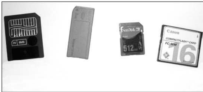
Figure 3.6 Several Popular Memory Cards: Smart Media, Sony Memory Stick, Compact Flash, and SD Memory
