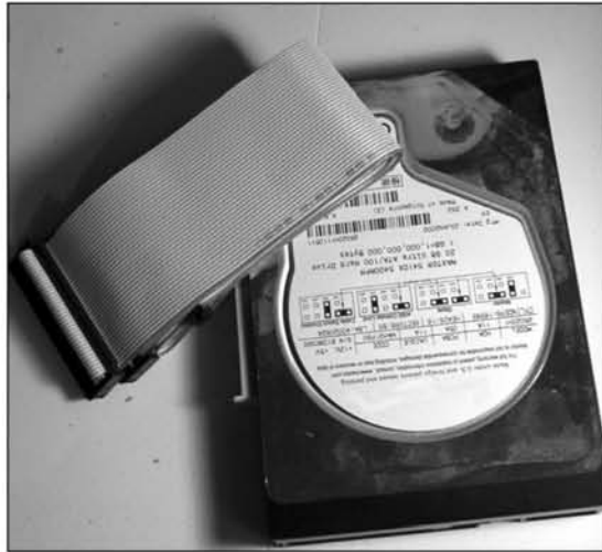
Figure 3.2 An Internal Hard Drive and ATA Cable for Connecting It to the Motherboard of the PC
