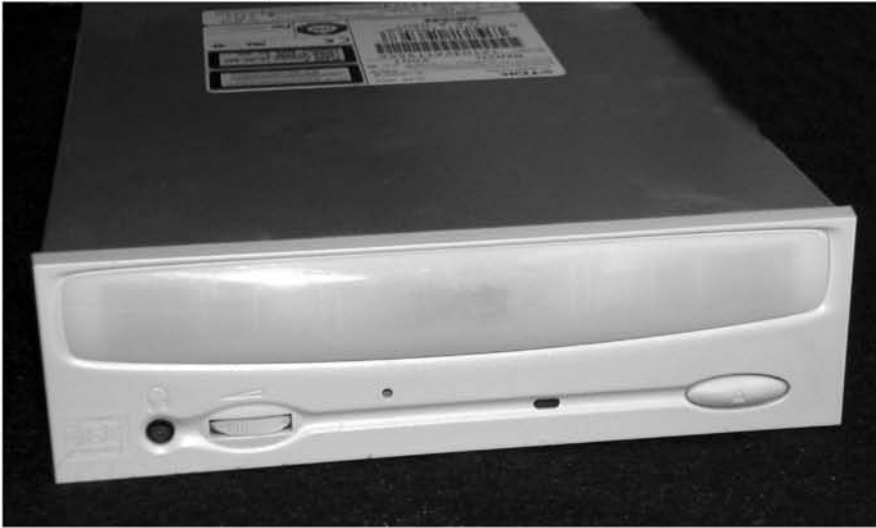
Figure 3.3 An Internal Optical Drive
