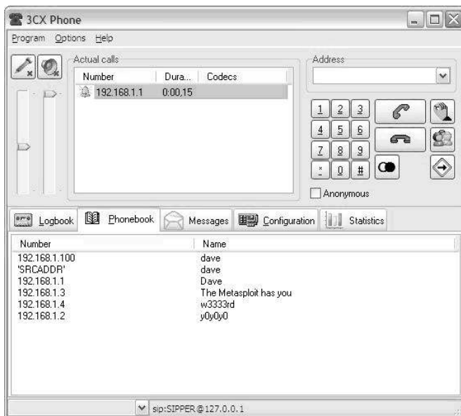
Figure 5.16 The VoIP SIP Invite Spoof Module Making a Softphone Ring
