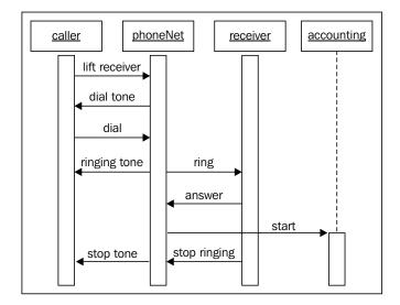
In a VoIP system, voice analog signals are converted into digital bits and then sampled and transmitted in the form of packets. To better visualize the difference between an ordinary phone and a VoIP phone, see the following flow:
