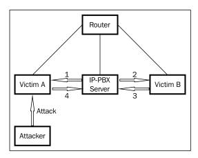
The components of the lab setup are as follows:
