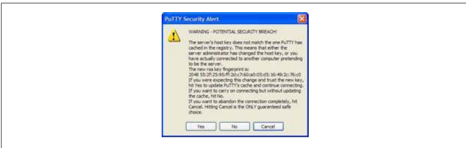
Figure 3-6. Warning message the victim sees once she connects to the SSH server, explaining that she previously connected to the SSH server and will receive a security host key mismatch warning from her SSH client
