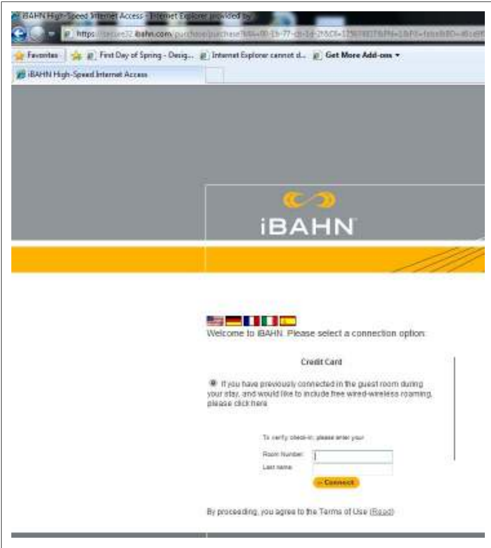
Figure 6-7. Room number and last name used to authenticate to the hotel's network
