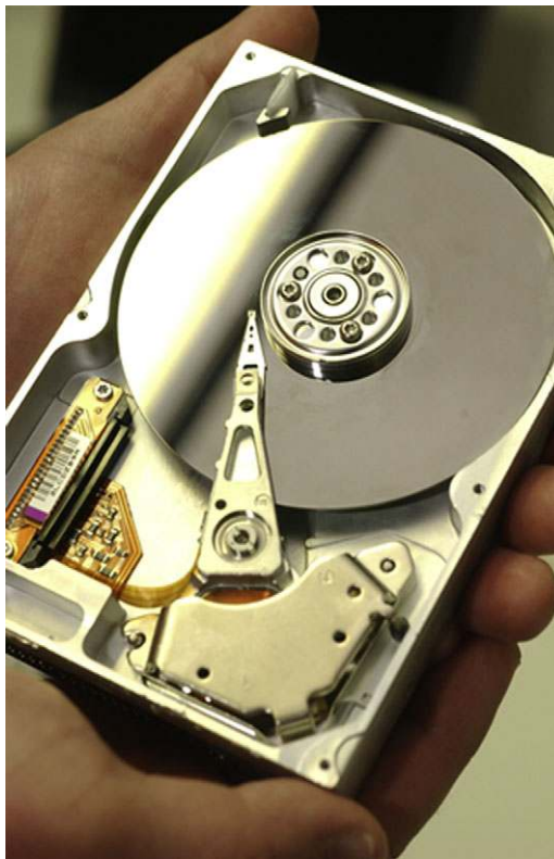
FIGURE 2.3 The inside of a typical magnetic drive.
