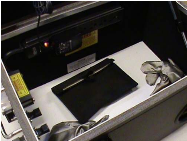
■ FIGURE 5.17 Internal container with isolation bag, cable, SIM card reader, and SIM card evidence holder.
