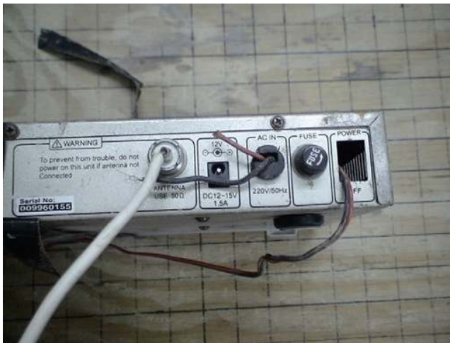
■ FIGURE 3.19 A modified Senao base station rigged to detonate an RCIED; 2006, AR Ramadi, Iraq. Photo taken by author Rich Watson.
