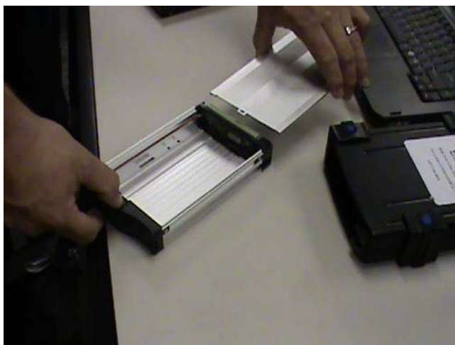
■ FIGURE 4.24 Drive cavity.
