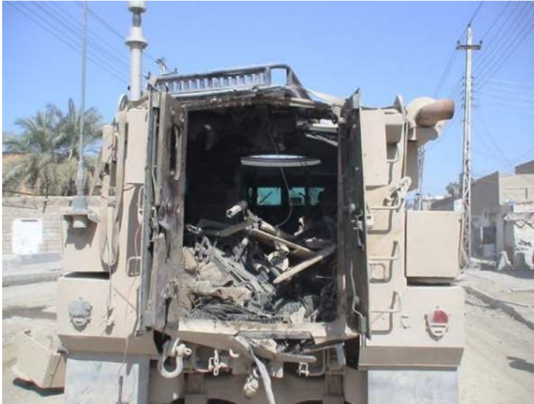
■ FIGURE 3.23 The rear of an EOD cougar that was destroyed when a VOIED was thought to be rendered safe and placed in the back of the vehicle. Unfortunately, one Marine EOD technician and one Navy Corpsman were killed in the detonation and one WIT member was severely injured; 2007, AR Ramadi, Iraq. Photo Courtesy of Marine SSG Daniel Bogart.
