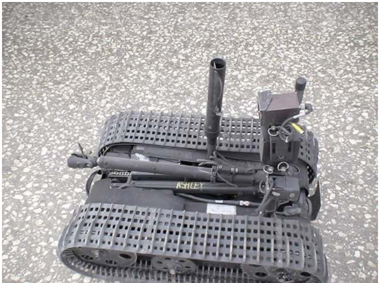
■ FIGURE 3.8 A Talon robot, 2006; AR Ramadi, Iraq. Photo taken by author Rich Watson.
