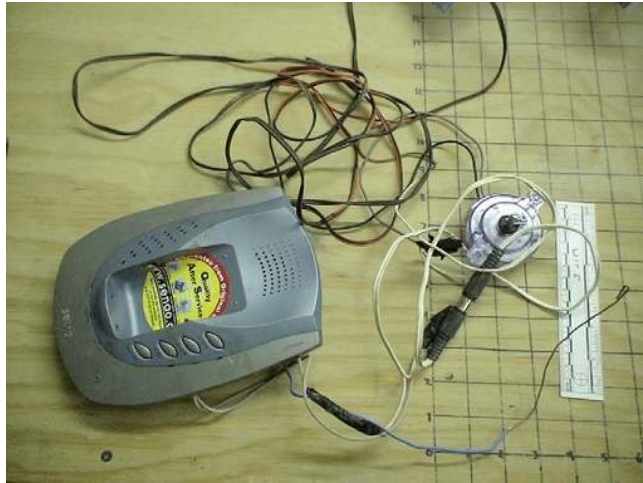
■ FIGURE 3.11 A Senao cordless telephone base station modified to remotely detonate an IED; 2006, AR Ramadi, Iraq. Photo taken by author Rich Watson.
