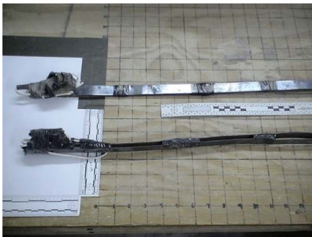
■ FIGURE 3.16 Pressure switches made from thin metal strips, black tape, foam, wires, and 9 v batteries; 2006, AR Ramadi, Iraq. Photo taken by author Rich Watson.
