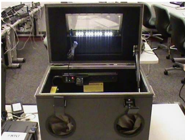
■ FIGURE 5.14 HTCI isolation chamber.
