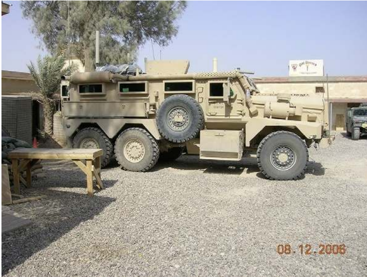
■ FIGURE 3.2 EOD Cougar commonly used to respond to IED scenes, 2006; AR Ramadi, Iraq. Photo taken by author Rich Watson.
