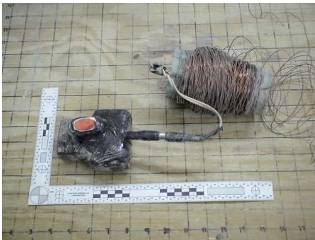
■ FIGURE 3.15 Typical initiating device with copper wire; 2006, AR Ramadi, Iraq. Photo taken by author Rich Watson.
